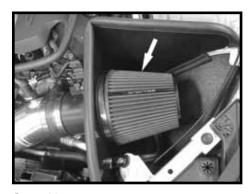
Step 13 Install the filter onto the MAFS velocity stack adapter and fasten it securely.
