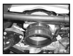
Step 11 Install the coupler onto the throttle body and secure with the provided hose clamp.
