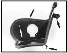
Step 8 Install the 2 plastic mounts onto the heatshield using the provided hardware. Install the third plastic mount onto the bracket then install the bracket onto the heatshield as shown. Then install the edge trim as shown.
