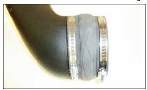
12. Install the provided hump coupler onto the intake tube with the hose clamps as shown.
