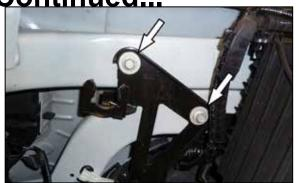
7. Remove the two bolts securing the air filter housing bracket to the inner fender and then remove the bracket from the vehicle.
