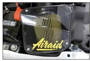
16. Install the AIRAID cover onto the air filter housing and secure with the provided hardware.
