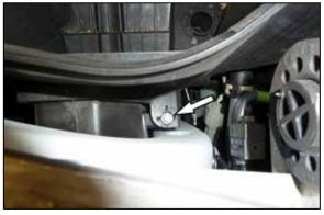
6. Remove the bolt securing the air filter housing and then remove the housing from the vehicle. NOTE: AIRAID, recommends that customers do not discard factory air intake.
