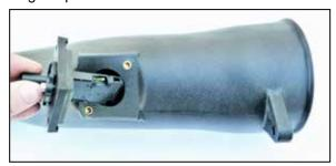
10. Install the mass sensor assembly into the AIRAID intake tube, be sure to install the sensor in the correct position so the opening of the sensor is pointer towards the filter end of the intake tube.
