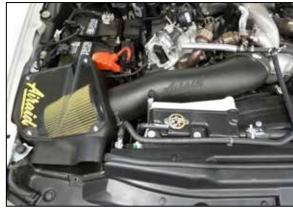
17. Double check your work! Make sure there is no foreign material in the intake path. Make sure all clamps, hoses, bolts, and screws are tight. Double check the hood clearance! Reconnect the negative battery cable!
