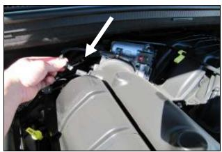
**2.** Disconnect the air temperature sensor from the air intake tube, just forward of the throttle body.
