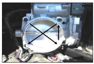
**6.** Reinstall the throttle body on top of the spacer using the four bolts and washers that are supplied with the kit. Tighten the bolts evenly to the vehicle manufacturers specifications, in a "X" pattern.
