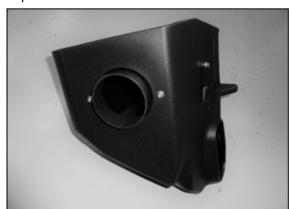
14. Install the filter adapter into the AIRAID filter housing and secure with the provided hardware.
