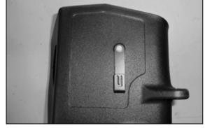
13. Install the provided bulk connector bracket onto the AIRAID air filter housing and secure with the provided hardware.
