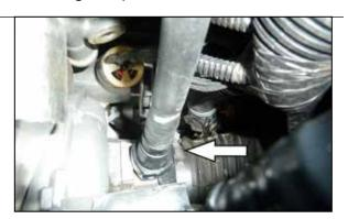
5.Loosen the hose clamp that secures intake tube to the turbo inlet.
