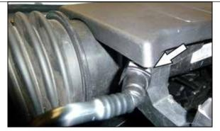
3. Depress the locking tab and then disconnect the CCV pipe from the plenum.
