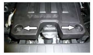
6. Remove the two bolts that secure the engine cover to the engine and then remove the cover from the vehicle. These bolts will be reused in a later step.
