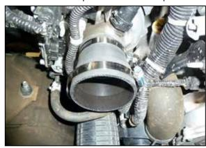
20. Install the provided straight coupler onto the turbo inlet and secure with the provided hose clamp.
