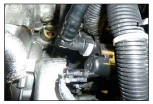
29. Connect the CCV tube to the solenoid and connect the electrical connection.
