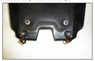
26. Using the factory bolts and the nuts provided, secure the two provided "Z" brackets to the engine cover as shown.
