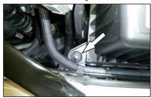
12. Remove the nut that secures the air filter housing to the mounting bracket. This nut will be reused in a later step.
