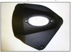
32.Install the AIRAID window into the AIRAID filter housing lid using the provided hardware.
