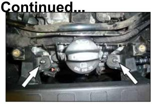
7. Remove the two nuts that secure the intake tube to the engine. Unhook the wiring harness from the intake tube and then remove the intake tube assembly from the vehicle. These nuts will be reused in a later step.
