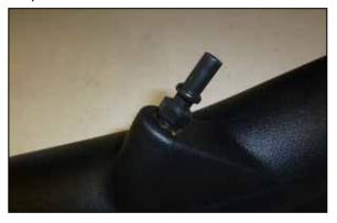
21. Install the provided quick connect fitting into the AIRAID intake tube.
