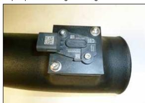
23. Install the mass air sensor assembly into the AIRAID intake tube and secure with the provided hardware as shown in the photo.
