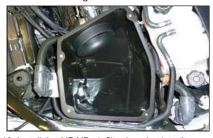
16. Install the AIRAID air filter housing into the vehicle and secure with the factory nut from step #12.
