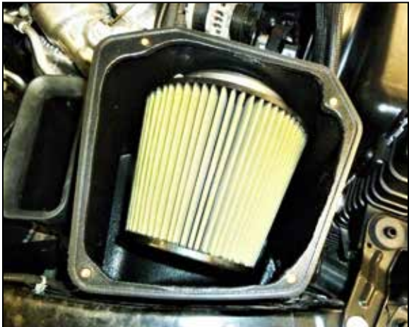
9. Slide the air filter onto the filter adapter and secure with the provided hose clamp.
