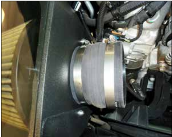
11. Install the provided hump coupler onto the filter adapter and secure with the provided hose clamp.
