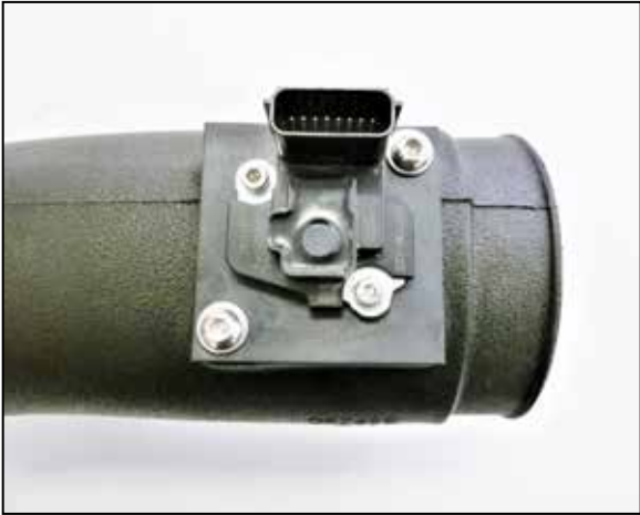
13. Install the mass air sensor assembly into the AIRAID intake tube and secure with the provided hardware. Be sure to install the sensor in the correct direction as shown. NOTE: 2024 model year vehicles and later have a different mass air sensor, the connector lays flat as compared to the sensor pictured.
