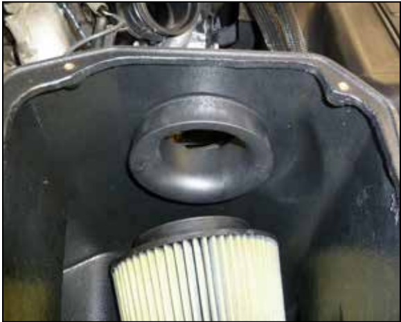
8. Install the filter adapter into the filter housing and secure with the provided hardware.
