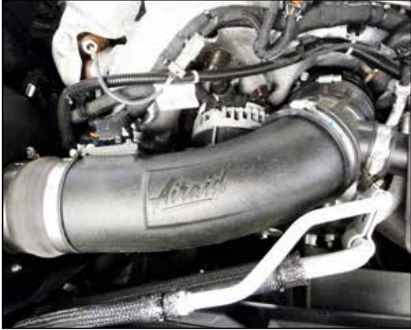
14. Install the intake tube assembly into the coupler at the filter adapter and then into the factory coupler, adjust the tube for best fit and secure with the hose clamps.
