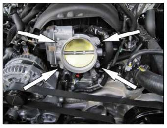
4. Remove the four bolts that secure the throttle body to the intake manifold. Pull the throttle body away from the intake manifold without disconnecting the wiring harness.
