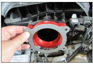
3. Install the AIRAID Spacer into the intake manifold with the supplied gasket on the throttle body side, as shown. \*Note: AIRAID spacer must be installed with bore protruding into intake manifold away from throttle body. Incorrect installation will hinder performance. Reference picture below for spacer orientation
