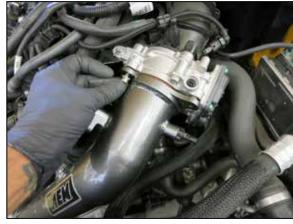
16. Secure the pipe to the throttle body with the hardware provided.
