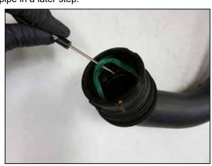
8. Remove the factory O-ring from the factory charge pipe.
