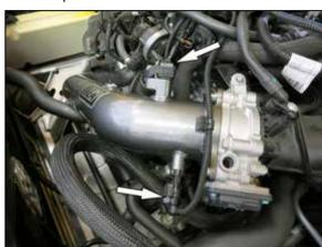
17. Reconnect the inlet temperature sensor and pressure sensor electrical connections.
