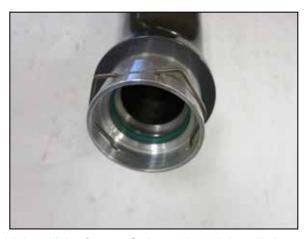
14. Install the factory O-ring and retaining clip into the AEM charge pipe as shown.
