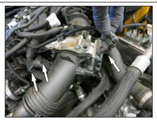
3. Disconnect the inlet air temperature sensor and pressure sensor electrical connections.
