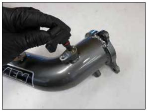
12. Install the pressure sensor into the AEM charge tube and secure with the provided hardware.
