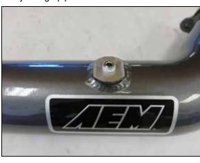
11. Install the 1/8npt pipe plug into the accessory port of the AEM charge pipe. Be sure to apply thread sealer to the plug before installation. Install the AEM decal as shown.
