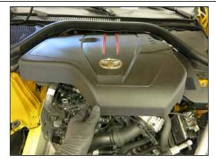
2. Lift up the engine cover to release it from the mounting grommets and then remove it from the vehicle. NOTE: THE INTAKE SYTEM HAS BEEN REMOVED FOR PHOTO'S.
