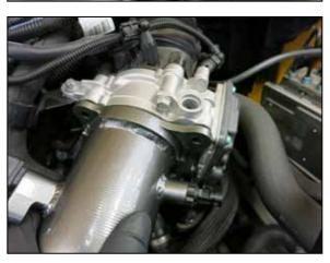
15. Install the AEM charge pipe onto the turbo inlet and throttle body. Push the tube onto the turbo until the retaining ring locks it into position while also aligning the top of the pipe with the throttle body.
