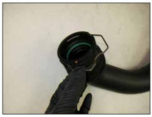
7. Remove the retaining clip from the stock charge pipe and set aside to be used with the AEM charge pipe in a later step.
