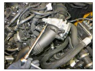
4. Remove the three bolts that secure the factory charge tube to the throttle body.
