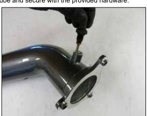
13. Install the inlet air temperature sensor into the AEM charge pipe.
