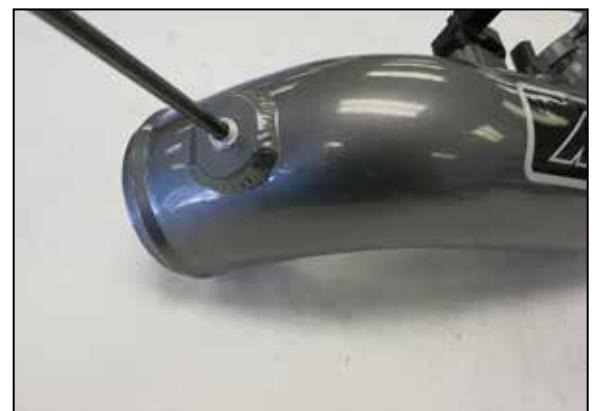
16. Install the 1/8npt pipe plug into the AEM charge pipe as shown. **NOTE: Be sure to use pipe sealant on the threads.**
