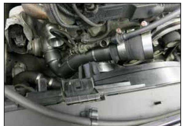
17. Install the step hose onto the lower charge tube section but do not tighten the clamp at this time. Install the lower tube section onto the turbo outlet, push the pipe on until the locking ring "clicks" into the locking groove.
