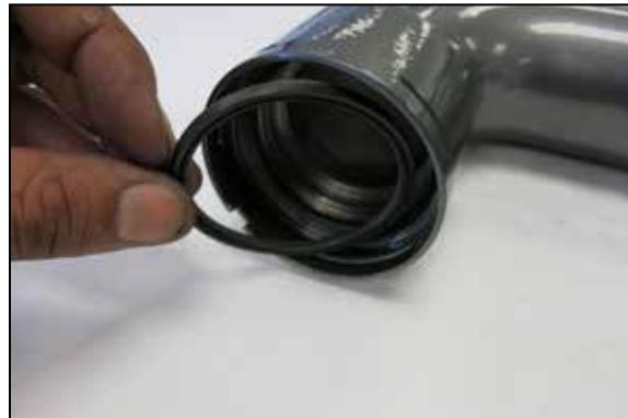
13. Install the factory O-ring into the AEM charge tube.
