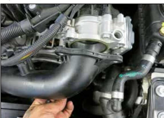
7. Using a T30 torx bit remove the three bolts that secure the charge tube to the throttle body.
