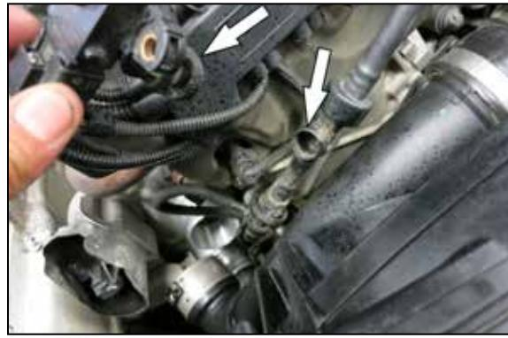
9. Disconnect the vacuum switch from the ccv line as shown to allow clearance for the charge pipe to be removed.
