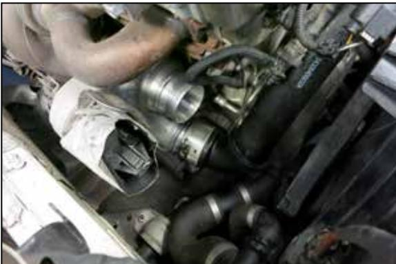
5. Loosen the clamp and then remove the intake tube from the turbo inlet.
