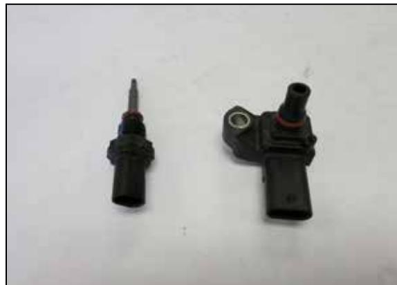
11. Remove the temperature sensor and pressure sensor from the factory charge tube.
