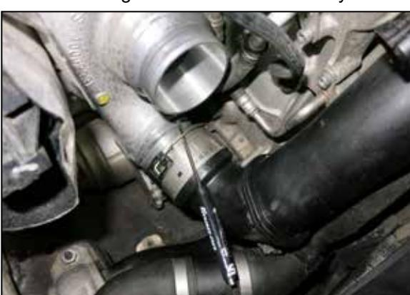
8. Using a flat blade screwdriver, unlock the clip that locks the charge pipe to the turbo outlet. Remove the charge tube assembly from the vehicle.
