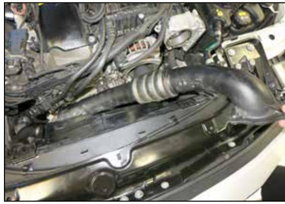
10. Remove the charge tube assembly from the vehicle.
