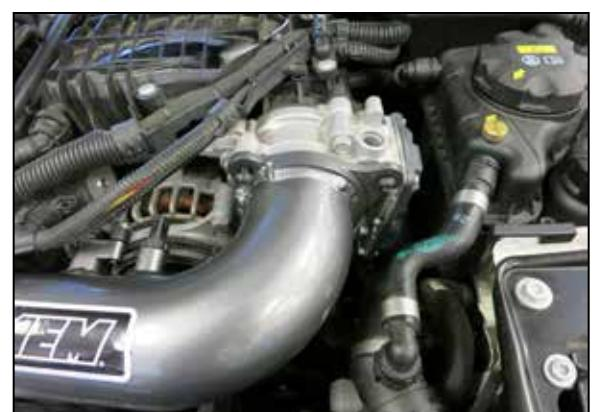
18. Install the upper AEM charge pipe into the coupler and then align with the throttle body, Secure the pipe to the throttle body with the factory bolts.
