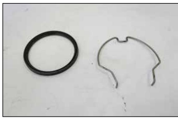
12. Remove the O-ring and locking clip from the factory charge pipe.
