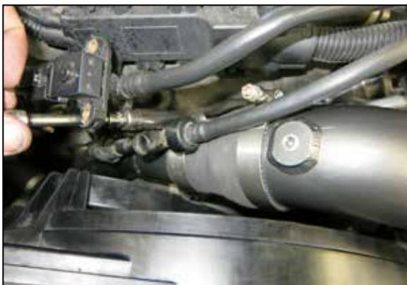
19. Align the lower pipe and step coupler for best fit and then tighten the hose clamps.
