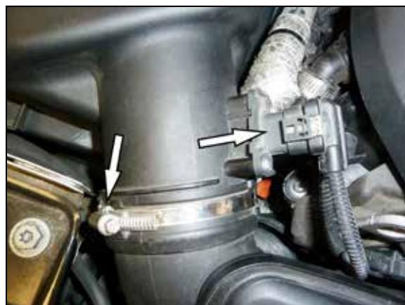
23. Reconnect the mass air sensor electrical connection and connect the intake tube to the air filter housing and secure with the factory hose clamp.
