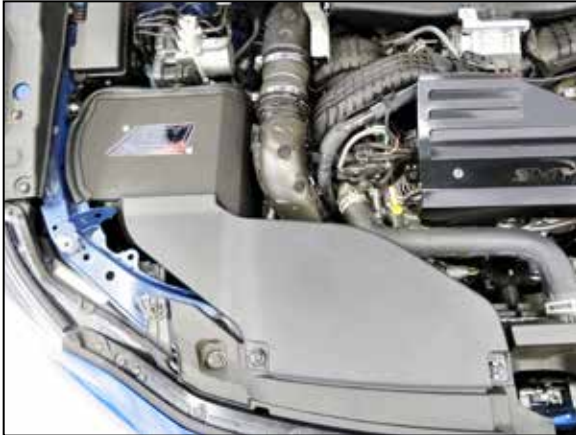
23. Reinstall the fresh air intake duct into the heat shield and secure with the factory mounting pins.
