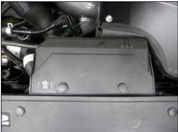
22. Install the fresh air intake duct and secure with the factory retaining clips.
