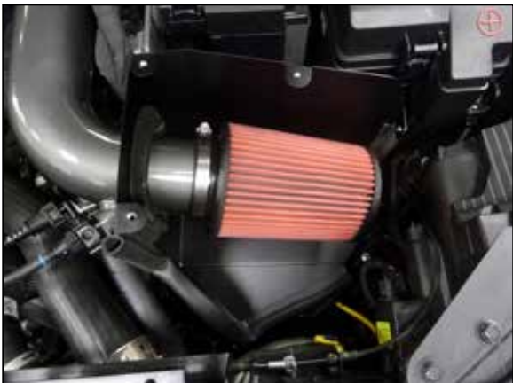
19. Install the AEM air filter onto the intake tube and secure with the provided hose clamp.
