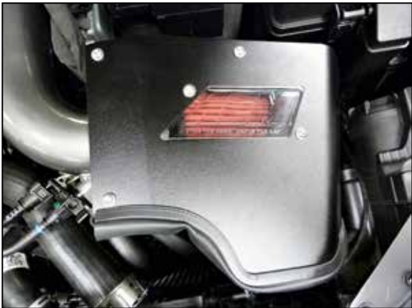
21. Install the lid onto the heat shield and secure with the provided hardware.
