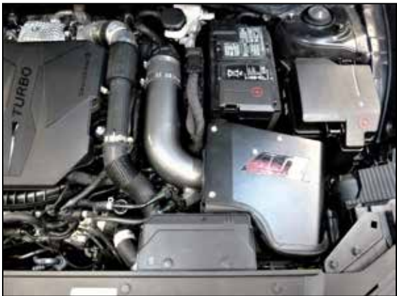
22. Install the fresh air intake duct and secure with the factory retaining clips.
