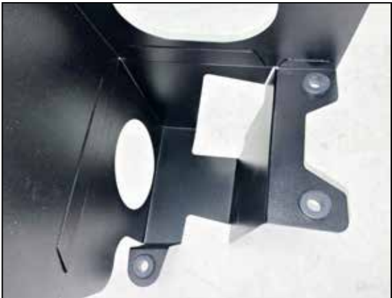
5. Install the provided grommets into the heat shield as shown.
