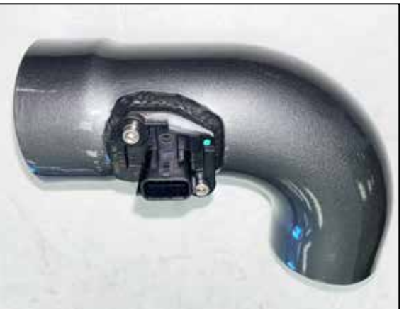
12. Remove the mass air sensor from the factory air filter housing and install it into the AEM intake tube and secure with the provided hardware.
