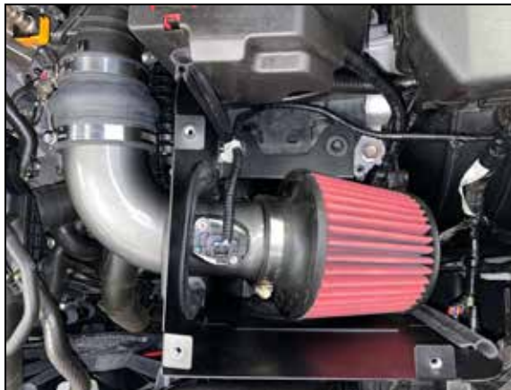
14. Install the air filter onto the intake tube and secure with the provided hose clamp.
