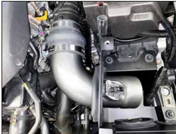
13. Install the AEM intake tube through the heat shield and into the coupler. Secure the coupler with the provided hose clamp.
