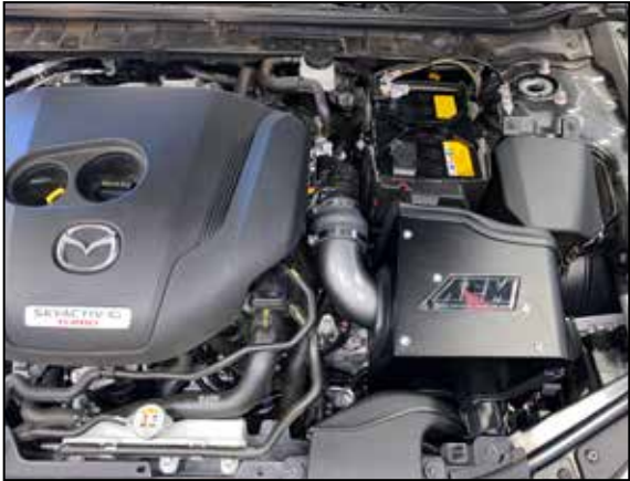
16. Install the heat shield lid onto the heat shield using the provided hardware.
