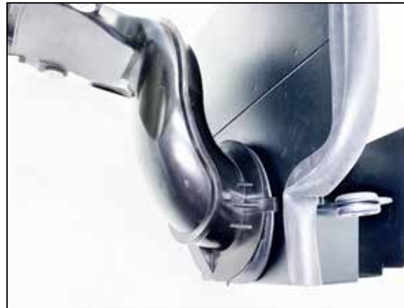
9. Install the fresh air duct into the AEM heat shield.
