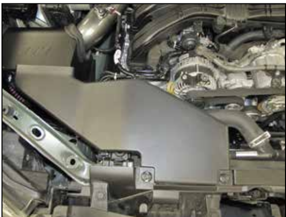
23. Install the fresh air intake duct into the heat shield and then secure with the factory retaining pins.
