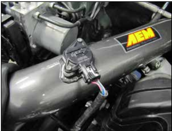
22. Reconnect the mass air sensor electrical connection.
