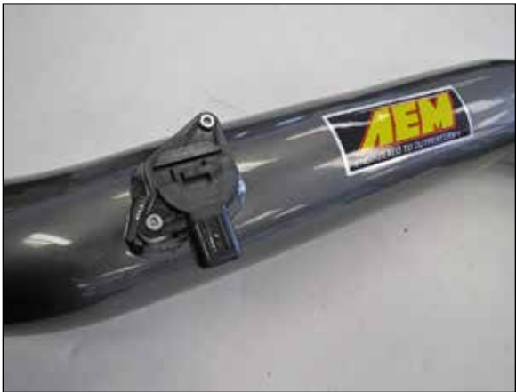
15. Install the mass air sensor into the AEM® intake tube and secure with the provided hardware.
