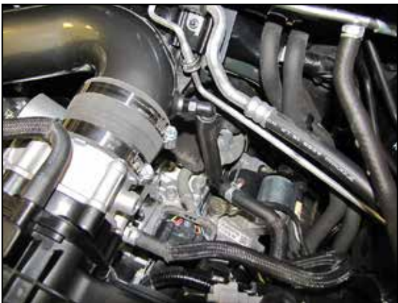
21. Adjust the tube for best fit and then secure with the provided hose clamps.
