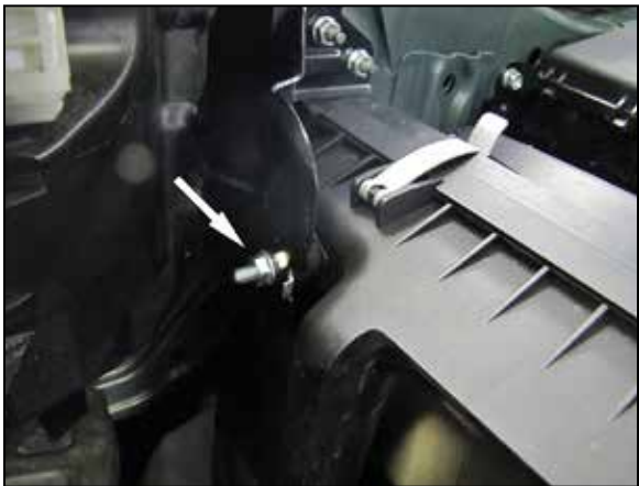
9. Remove the nut that secures the air filter housing to the bracket attached to the fender.
