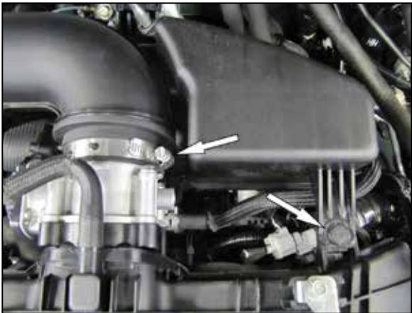
5. Remove the clip that secures the intake plenum and loosen the hose clamp at the throttle body.
