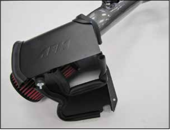
18. Install the AEM® intake tube through the heat shield and install the AEM® air filter onto the tube and secure with the provided hose clamp.
