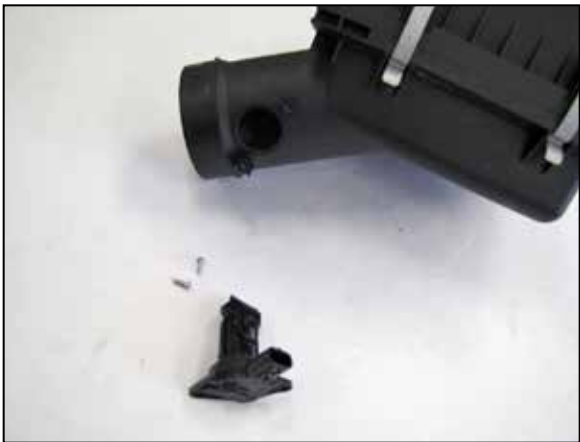
14. Remove the mass air sensor from the factory air filter housing.
