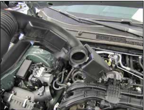
7. Remove the factory intake tube from vehicle.
