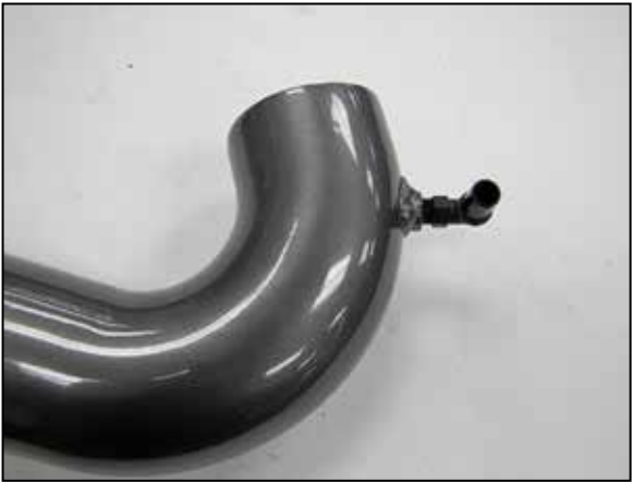
16. Install the 90° vent fitting into the AEM® intake tube as shown. NOTE: Plastic NPT fittings are easy to cross thread. Install the vent fitting "hand" tight, then turn it two complete turns with a wrench.
