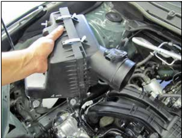
10. Remove the complete air filter housing assembly from the vehicle. NOTE: AEM recommends that customers do not discard factory air intake.
