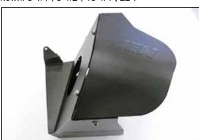
10. Attach the heat shield lid using the provided hardware.
