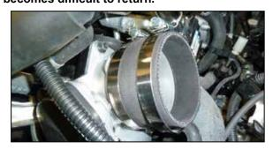
8. Install the provided coupler onto the throttle body and secure with the provided hose clamp.
