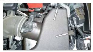
2. Disconnect the mass air sensor electrical connector and then disconnect the wiring harness from the air filter housing.
