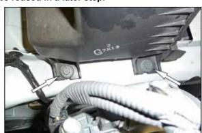
7. Remove the two bolts that secure the air filter housing to the frame rail, then remove the air filter housing. NOTE: These bolts will be reused later. NOTE: AEM recommends that customers do not discard factory air intake.
