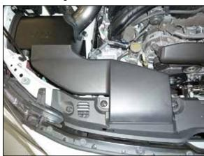
24. Reinstall the factory fresh air intake duct and secure with the factory hardware.
