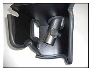
12. Install the AEM® intake tube trough the heat shield, then remove the mass air sensor from the factory housing and install it into the AEM® intake tube using the provided hardware.
