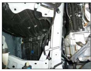
15. Position the mass air sensor wiring pigtail along the frame as shown.
