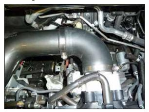
20. Align the intake tube for best fit and then secure the coupler hose clamps.
