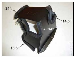
11. Install the edge trim onto the heat shield as shown.
