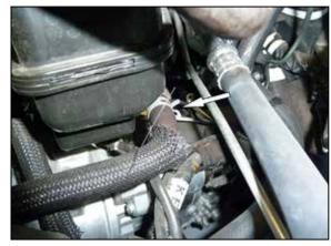
3. Release the spring clamp securing the vent hose to the intake plenum and then disconnect the hose from the plenum.
