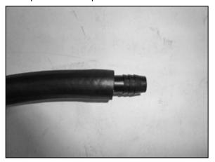
21. Install the provided hose union into the provided crank case vent hose as shown.
