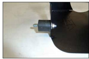
10. Install the provided rubber mounted stud onto the heat shield using the factory nut.
