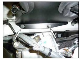
17. Secure the heat shield to the frame with the factory air filter housing mounting bolts.
