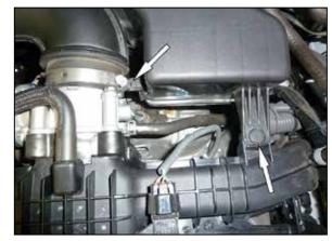
4. Remove the clip that secures the intake plenum to the manifold and then loosen the hose clamp that secures the intake tube to the throttle body.
