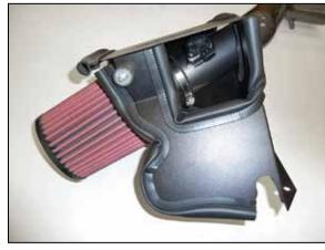
13. Install the AEM® air filter onto the intake tube and secure with the provided hose clamp.
