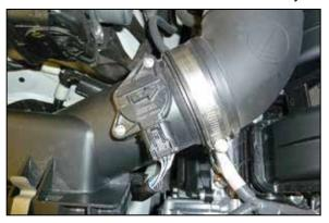
5. Loosen the hose clamp securing the intake tube to the air filter housing and disconnect the mass air sensor electrical connection.
