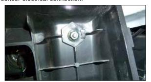
6. Release the air filter housing clips and remove the housing half and factory air filter. Remove the air filter housing retaining nut. **NOTE: This nut will be reused in a later step.**
