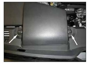
2. Remove the two clips that secure the fresh air intake duct and then remove the duct from the vehicle.
