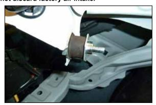
8. Remove the factory air filter housing mounting stud. **NOTE: The Mounting nut will be reused in a later step.**
