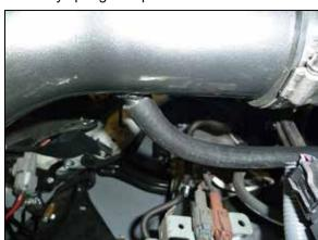
23. Connect the open end of the crank case vent hose to the fitting on the AEM® intake tube.
