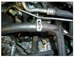
22. Install the crank case vent hose assembly into the factory crank case vent hose and secure with the factory spring clamp.
