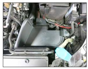
9. Install the AEM heat shield onto the factory air box mounting studs. Soapy water may be used to help the grommets engage with the studs.
