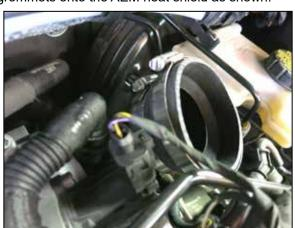
7. Install the provided coupler and hose clamps onto the turbo with the small end towards the turbo inlet. Tighten the turbo-side hose clamp to 30in-lb.
