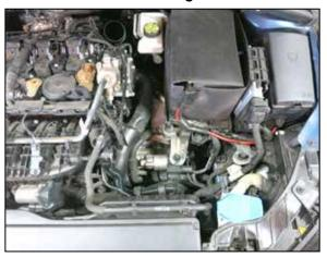
5. Remove the stock air box and intake hose assembly from the vehicle by pulling upwards to disengage the three rubber grommets. Lift the hose side first and maneuver the box towards the rear, clearing the cold air inlet.
