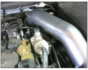
11. Lower the AEM intake tube bracket onto the rubber mount, between the washer and rubber mount, and insert the tube into the coupler. Do not tighten the mount or coupler at this time.
