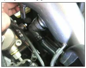
10. Position the AEM intake tube in the engine bay and connect the small vacuum hose to the small nipple. Move the large air injection hose behind the AEM heat shield and connect it to the AEM intake tube. Soapy water should be used to help installation. Note: Not all models have this large hose. Install the included blind plug (8-215) in its place. On vehicles that the factory vacuum line is too short, use the provided union and vacum line to complete the connection.
