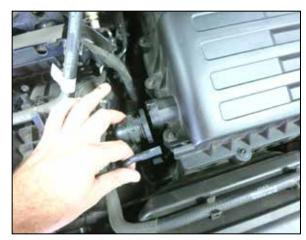
4. Remove small vacuum line from the stock air box. Remove the large air injection hose by depressing the ribber parts of the collar. **Note: Not all models will have this large hose.**
