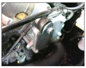
8. Install the provied rubber mount onto the side of the engine. Loosely install the provided washer and nut onto the tuber mount.
