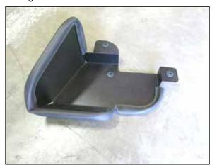
6. Install the provided edge trim and rubber grommets onto the AEM heat shield as shown.
