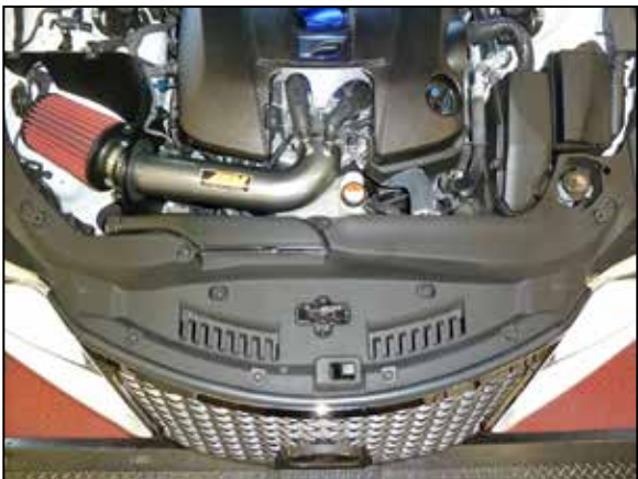
20. Reinstall the core support shroud and secure with the factory push pins.
