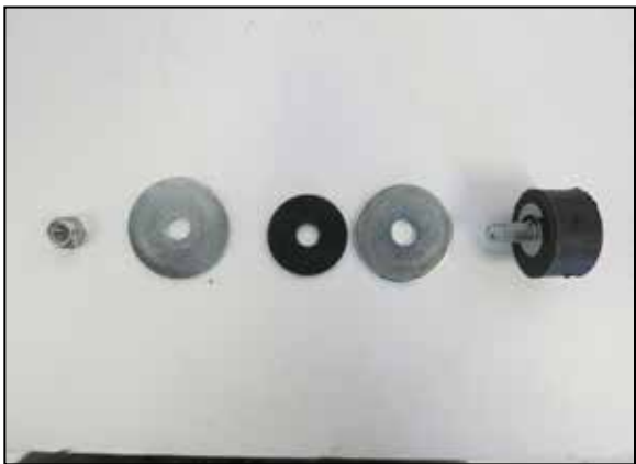
9. Remove the two-factory air filter housing mounting grommets.
