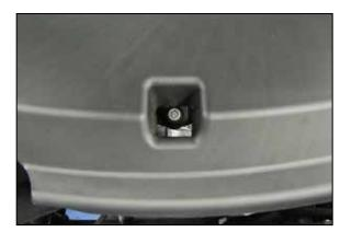
4. Remove the front center bolt securing the intake plenum to the engine and remove the intake plenum from the vehicle.
