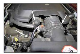
2. Loosen the hose clamp that secures the intake hose to the air filter housing. Using a screwdriver, unlock the small clamp that secures the vent line to the connector and then disconnect the vent line. Remove the bolt securing the intake plenum to the engine.
