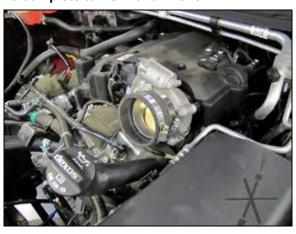
16. Install the provided coupler (08186) onto the throttle body and secure with the provided hose clamp.
