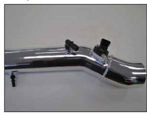
15. Install the  $90^{\circ}$  vent fitting into the K&N® intake tube as shown.
