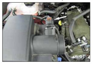
5. Release the red locking tab and then disconnect the mass air sensor electrical connection and unhook the harness from the air filter housing.
