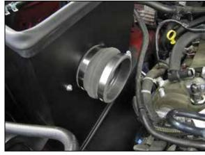
17. Install the provided hump coupler (08699) onto the heat shield and secure with the provided hose clamp
