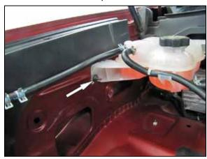
11. Remove the nut that secures the coolant reservoir to the inner fender.
