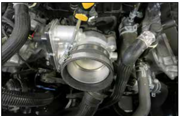
13. Install the provided straight coupler onto the throttle body and secure with the provided hose clamp.
