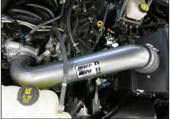
17. Install the Intake tube into the coupler at the throttle body and then into the coupler at the filter adapter, adjust the tube for best fit and secure with the provided hose clamps.
