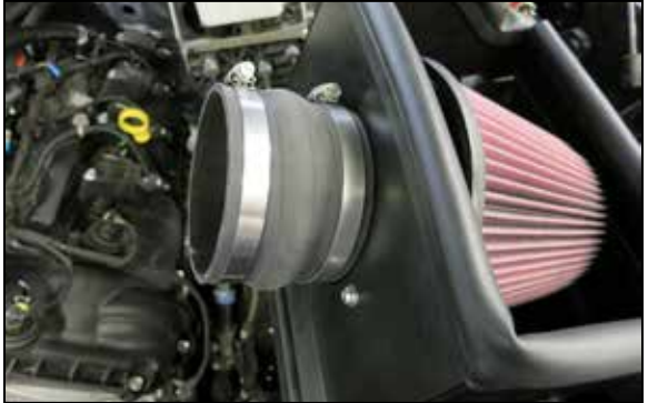
15. Install the provided hump hose onto the filter adapter and secure with the provided hose clamp.
