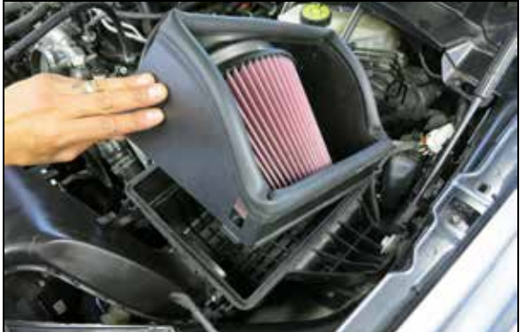
14. Install the Heat shield/Filter assembly onto the lower air filter housing and secure with the factory retaining clips.
