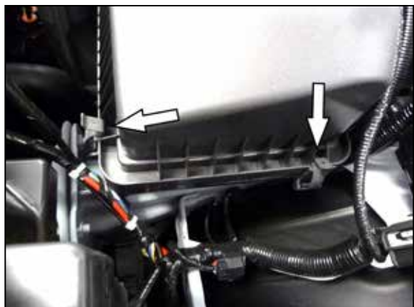
4. Release the two spring clips that secure the air filter housing lid, remove the lid and factory air filter. NOTE: K&N Engineering, Inc., recommends that customers do not discard factory air intake.
