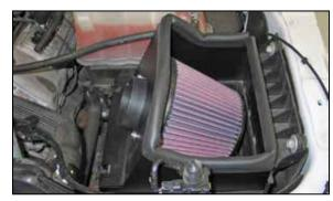
13. Install the K&N® filter/heat shield assembly and secure with the two remaining factory upper air box retaining clips.
