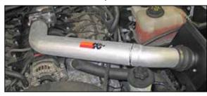
19. Install the K&N® intake tube into the silicone hose at the air filter and then into the silicone hose at the throttle body and secure with the provided hose clamps.
