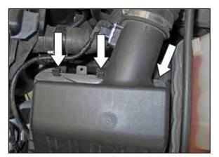
3. Release the three upper air box retaining clips.
