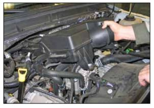
8. Unhook the heater hose clip from the intake plenum and then remove the plenum from the vehicle.
