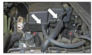
6. Disconnect the crank case vent line and EVAP vent line from the intake plenum.
