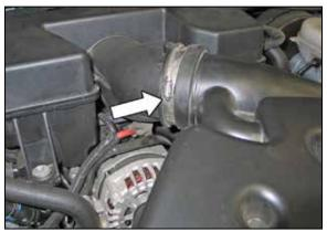
4. Loosen the hose clamp securing the intake tube to the intake plenum.
