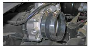
14. Install the provided silicone hose (08630) onto the throttle body and secure with the provided hose clamp.
