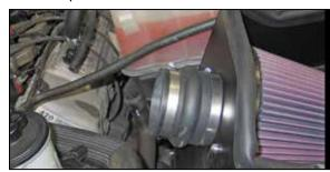
15. Install the provided silicone hump hose (5-576) onto the filter adapter and secure with the provided hose clamp.
