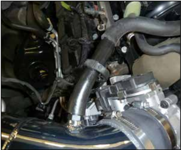
17. Remove the short section of the factory CCV hose and install the straight section provided. Connect the CCV hose to the fitting installed into the K&N intake tube.
