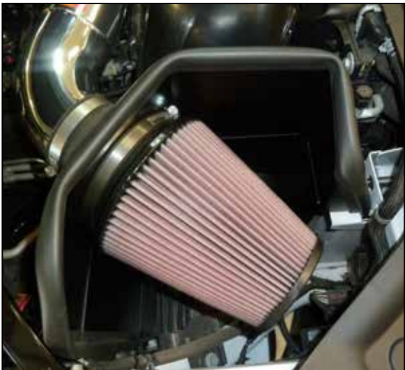
20. Install the K&N air filter and secure with the provided hose clamp.
