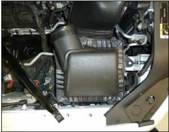
6. Pull the factory air filter housing straight up and remove it from the vehicle. NOTE: K&N Engineering, Inc., recommends that customers do not discard factory air intake.
