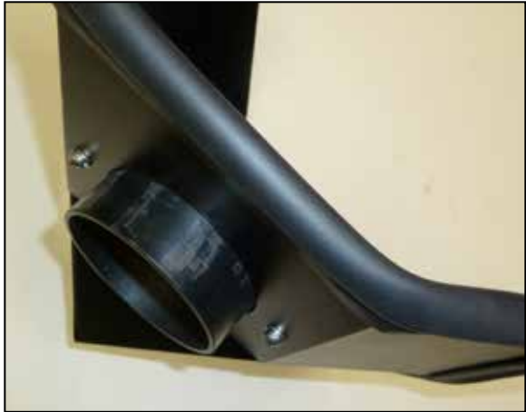
8. Install the filter adapter into the heat shield and secure with the provided hardware.
