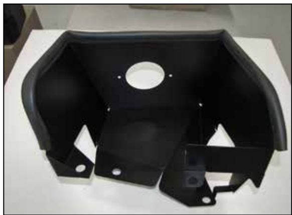
4. Install the provided edge trim onto the heat shield as shown. NOTE: Some trimming of the edge trim will be necessary.
