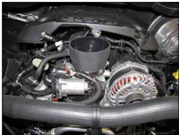
8. Install the provided coupler (08497) onto the throttle body and secure with the provided hose clamp.
