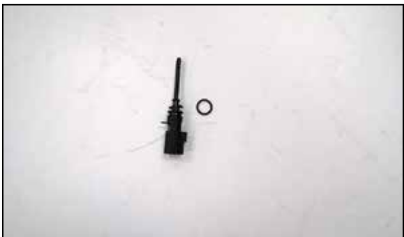
10. Remove the inlet air temperature sensor from the factory intake tube and remove the O-ring from the sensor.
