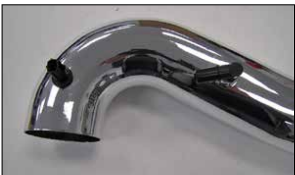
11. Install the inlet air temperature sensor into the K&N intake tube using the provided grommet. Install the 90° NPT fitting onto the K&N intake tube as shown. NOTE: Plastic NPT fittings are easy to cross thread. Install the vent fitting “hand” tight, then turn it two complete turns with a wrench.
