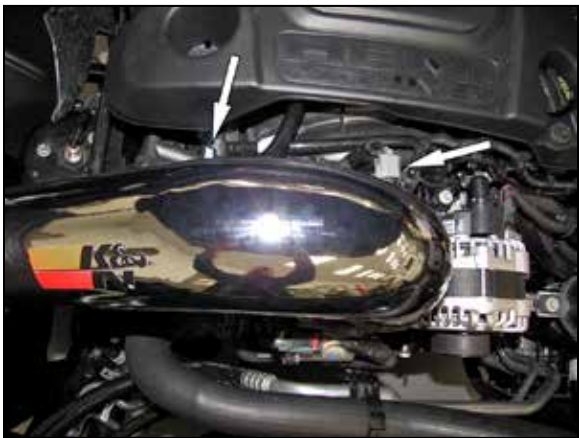
13. Connect the crank case vent line and inlet air temperature sensor electrical connection.
