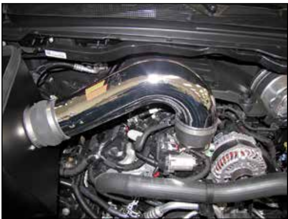
12. Install the K&N intake tube into the coupler at the heat shield and then into the coupler on the throttle body, adjust the tube for best fit and then secure with the provided hose clamps.
