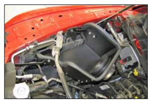
14. Install the heat shield into the vehicle and secure with the factory bolts removed in the previous steps.
