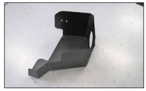
6. Install the heat shield side wall onto the heat shield and secure with the provided hardware.
