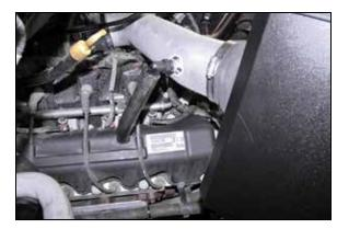
21. Install the provided crank case vent hose onto the valve cover port and then connect the open end to the fitting installed into the K&N® intake tube.
