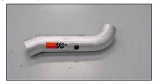
15. Install the provided grommet into the K&N® intake tube as shown.
