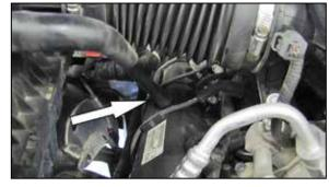
3. Disconnect the crank case vent hose from the valve cover fitting and then lift up and remove the air filter housing and intake tube to remove it from
