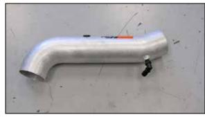
16. Install the 90° NPT fitting into the K&N $^{\rm 8}$  intake tube as shown.
