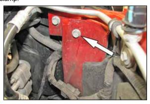
12. Remove the core support bolt shown. **NOTE: This bolt will be reused in a later step.**
