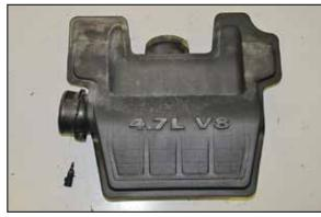
17. Remove the inlet air temperature sensor from the factory air filter housing.
