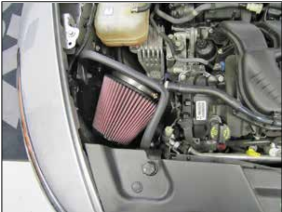
13. Install the heat shield assembly into the vehicle and secure with the hardware removed in step #6. NOTE: Do not completely tighten at this time.
