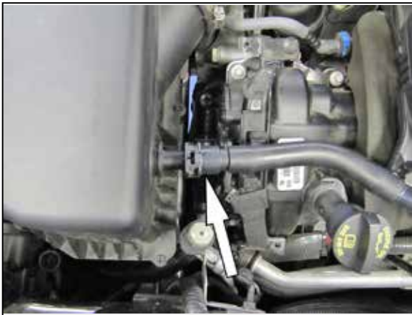
3. Disconnect the crank case vent hose from the air filter housing.
