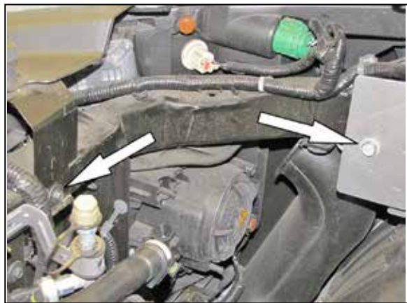
6. Remove the two factory bolts shown. NOTE: These bolts will be reused in a later step.
