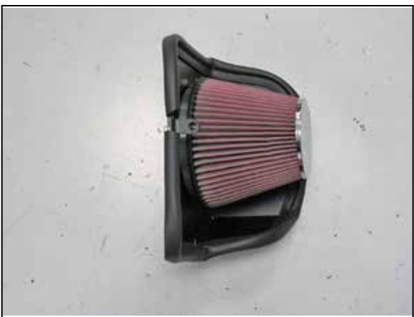
12. Install the K&N® air filter onto the filter adapter and secure with the provided hose clamp.
