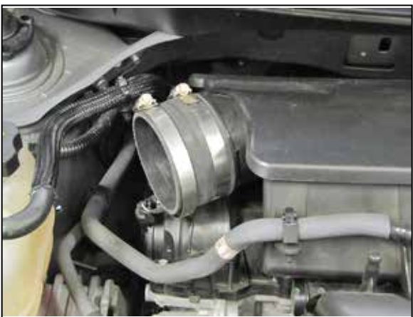
14. Install the provided coupler hose (08690) onto the intake plenum and secure with the provided hose clamp.
