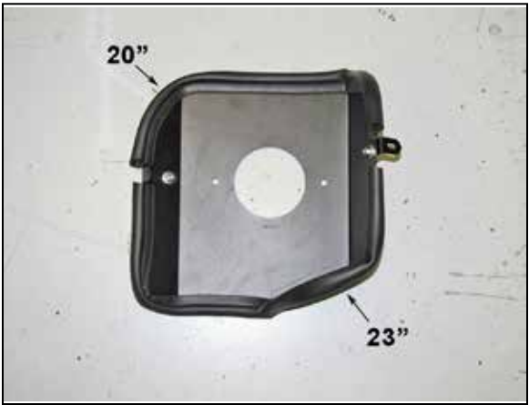
10. Install the provided edge trim onto the heat shield as shown.
