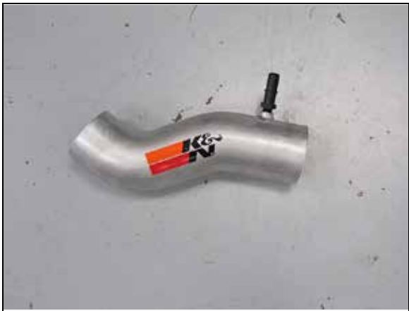
15. Install the provided quick disconnect fitting into the K&N® intake tube as shown. NOTE: NPT fittings are easy to cross thread. Install the vent fitting "hand" tight, then turn it two complete turns with a wrench.
