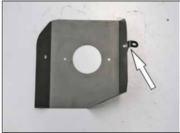
7. Install the heat shield mounting bracket (064323) onto the heat shield as shown using the provided hardware.
