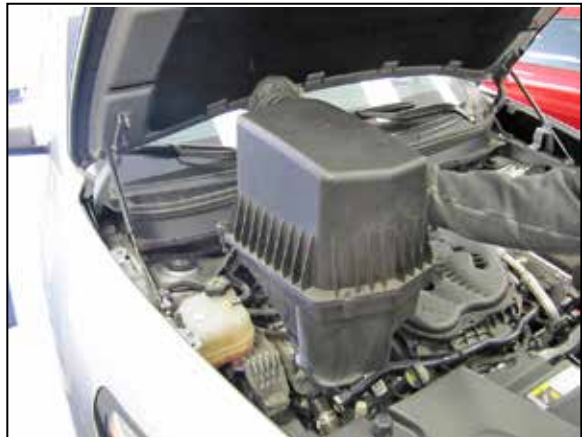
5. Lift up the air filter housing to dislodge it from the mounting grommets and then remove the complete air filter housing assembly from the vehicle. NOTE: K&N Engineering, Inc., recommends that customers do not discard factory air intake.
