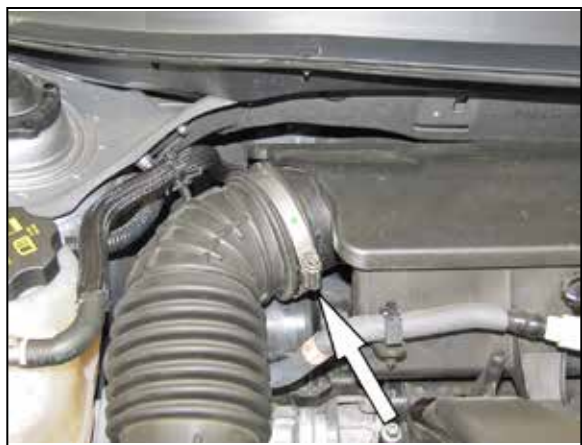
4. Loosen the hose clamp that secures the intake tube to the intake plenum.
