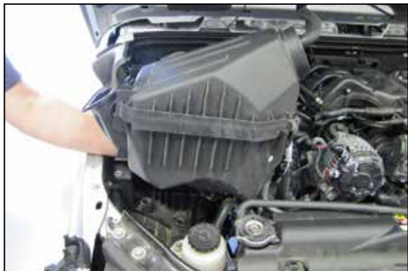
8. Lift up and remove the air filter housing from the vehicle NOTE: K&N Engineering, Inc., recommends that customers do not discard factory air intake.
