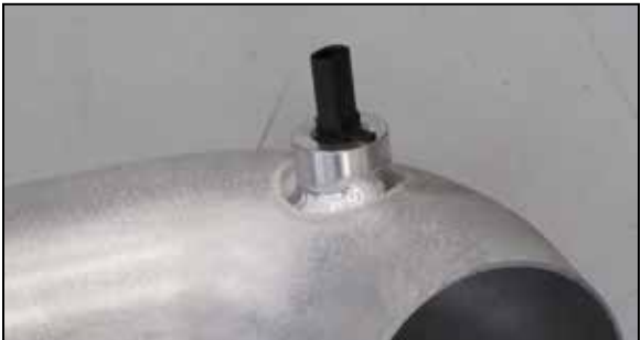
28. Install the inlet air temperature sensor into the K&N® intake tube as shown. NOTE: Align the tab on the sensor with the line on the sensor mount then rotate clockwise to lock into position.
