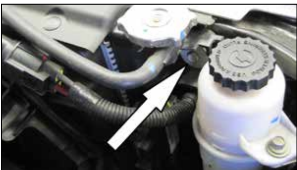
10. Remove the bolt shown that secures the radiator to the core support. NOTE: This bolt will be reused in a later step.
