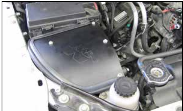
22. Install the K&N® filter lid and secure with the provided hardware. NOTE: Install the bolt into the bracket 1st.
