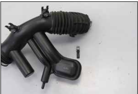
27. Remove the inlet air temperature sensor from the factory intake plenum as shown. NOTE: Use caution working with the inlet air temperature sensor as it is very fragile.
