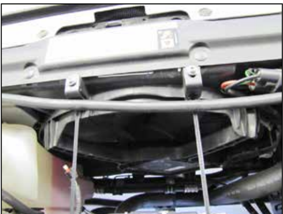
30. Install the tie wrap equipped brackets onto the factory intake tube mounting locations on the fan shroud using the provided hardware. Then secure the coolant over flow hose with the tie wraps.
