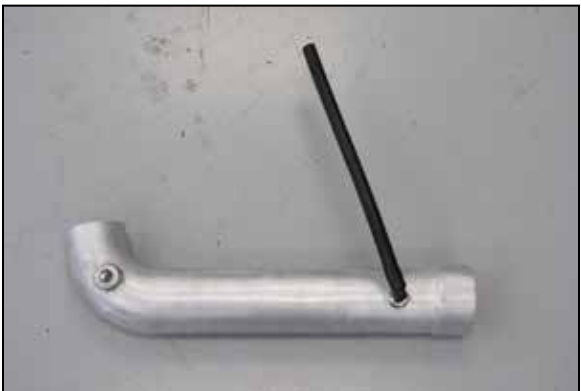
26. Install the provided crank case vent hose onto the fitting as shown
