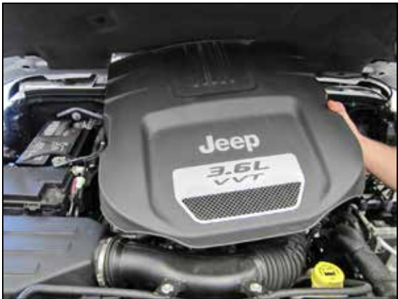
2. Lift up and remove the engine cover.
