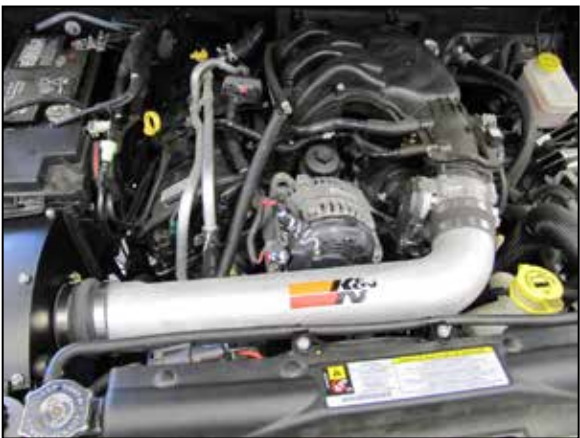
31. Install the K&N® intake tube into the silicone hose at the filter adapter and then into the hose at the throttle body, then secure with the provided hose clamps.
