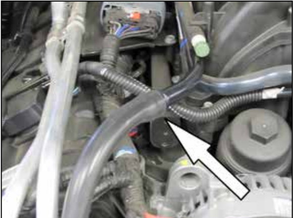
32. Connect the open end of the crank case vent hose to the factory crank case vent tube as shown.
