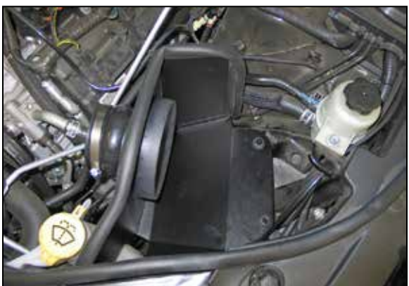
15. Set the heat shield into the vehicle so that the mounting grommets slide over the factory air box mounting studs.
