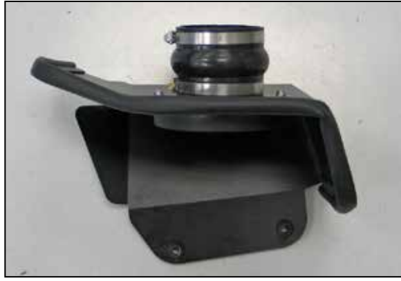
14. Install the provided silicone hump hose (084057) onto the filter adapter and secure with the provided hose clamp.
