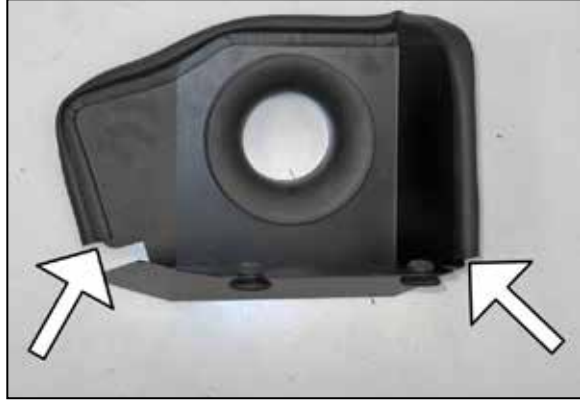
13. Install the provided edge trim onto the heat shield as shown. NOTE: Some trimming of the edge trim will be necessary.
