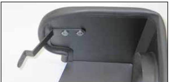
15. Install the heat shield mounting bracket (083127A) onto the heat shield using the provided hardware. NOTE: Do not completely tighten at this time.
