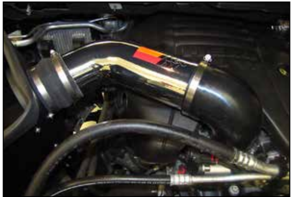
25. Install the K&N intake tube into the silicone hump hose and then into the silicone hose attached to the throttle body. Align the heat shield assembly for proper fitment. Tighten the heat shield mounting bolts and hose clamps securing the intake tube.
