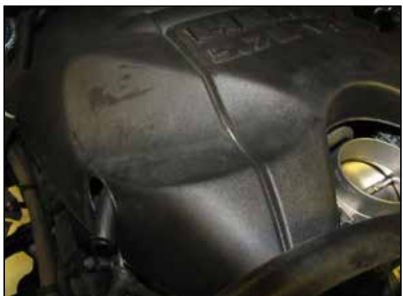
10. Reinstall the engine cover and position the CCV hose through the opening.
