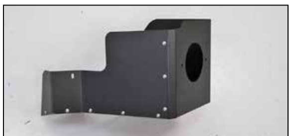
11. Some vehicles may have an AC line obstructing installation. Choose the appropriate heat shield wall for the AC line configuration and attach to the heat shield as shown using the provided hardware.
