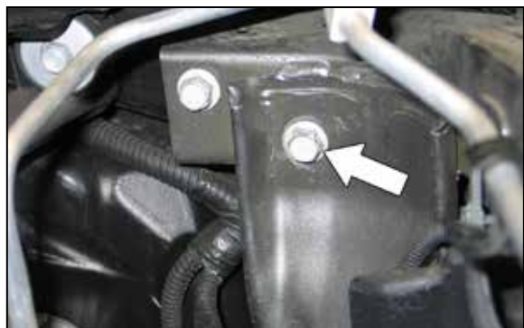
18. Remove the front fender mounting bolt shown. NOTE: This bolt will be used in a later step.
