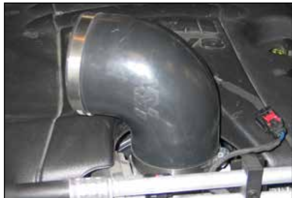
20. Install the provided silicone hose (084086-1) onto the throttle body and secure with the provided hose clamp.
