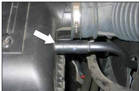
4. Disconnect the crank case vent hose from the air box.
