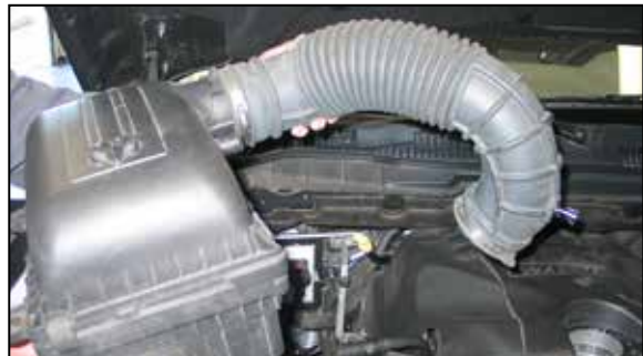
5. Disconnect the factory intake hose from the throttle body, then lift up the air box assembly and remove it from the vehicle. NOTE: K&N Engineering, Inc., recommends that customers do not discard factory air intake.
