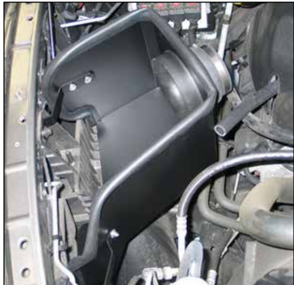
19. Install the heat shield assembly into the vehicle and secure with the bolts removed in steps #17 and 18. Do not completely tighten at this time.
