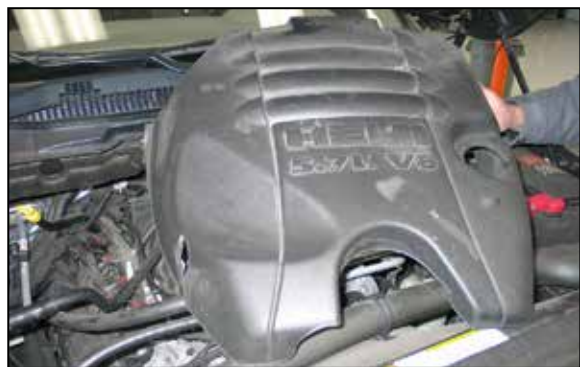
6. Lift up the engine cover to dislodge it from the mounting posts and then remove it from the vehicle.
