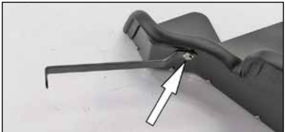
16. Install the heat shield mounting bracket (083103-1A) onto the heat shield using the provided hardware. NOTE: Do not completely tighten at this time. NOTE: When using the cut out heat shield wall, place the provided spacer between the bracket and heat shield and use the longer bolt.
