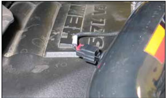
27. Connect the provided inlet temperature sensor extension into the factory wiring harness and then connect the other end to the inlet temperature sensor. NOTE: The vehicle manufacturer uses two different inlet air temperature sensor connections, choose the correct extension harness for the sensor provided by the manufacturer. Secure the harness with the provided tie wrap.
