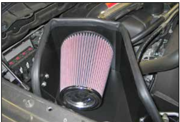
28. Install the K&N air filter and secure with the provided hose clamp.
