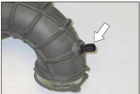
23. Remove the inlet air temperature sensor from the stock intake tube. NOTE: Use care removing the sensor as it is very fragile.
