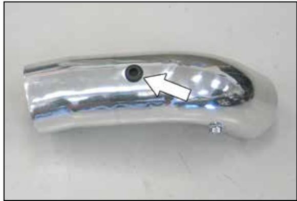
21. Install the provided grommet into the K&N intake tube as shown.
