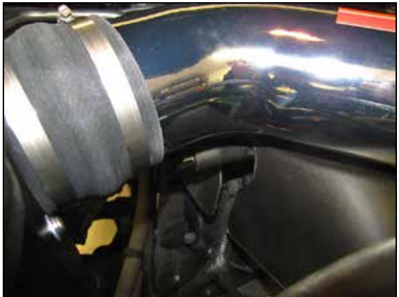
26. Connect the CCV hose to the 90deg. fitting installed into the K&N intake tube.
