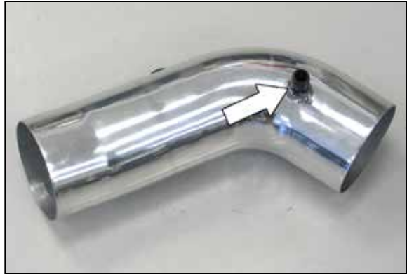
22. Install the 1/4 npt vent fitting into the K&N intake tube as shown. NOTE: NPT fittings are easy to cross thread. Install the vent fitting "hand" tight, then turn it two complete turns with a wrench.
