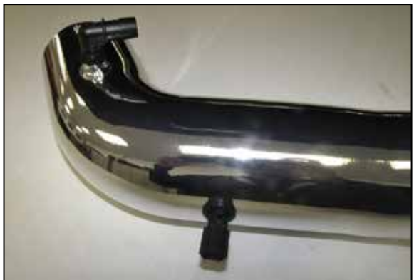
24. Install the inlet air temperature sensor into the grommet installed into the K&N intake tube as shown. NOTE: Use care while installing the inlet air temperature sensor as it is very fragile.
