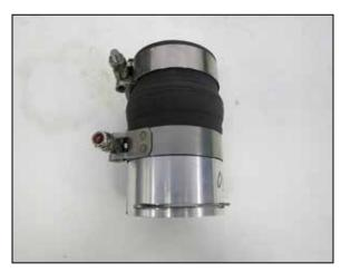
8. Install the hump coupler onto the K&N "Hot Side" inter cooler quick connector 088120 and secure with the provided hose clamp.
