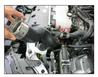
4. Remove the cold side charge tube from the vehicle.
