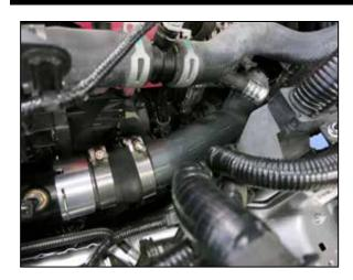
14. Install the K&N "Cold Side" charge tube into the coupler, then position the tube onto the engine inlet and push the tube onto the inlet until an audible "click" is heard as the retaining clip locks onto the inlet. Position the tube and coupler for best fit and then secure the hose clamps. Position the "Cold Side" charge tube for best fit and then secure the hose clamps.
