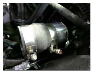
9. Install the "Hot Side" quick connector assembly onto the inter cooler as shown. Push the coupler onto the inter cooler until an audible "click" is heard as the retaining clip locks onto the inter cooler inlet.
