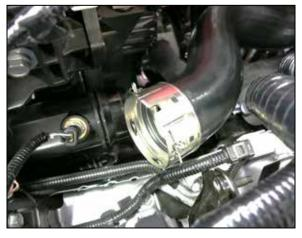
3. Pull the "Cold Side" charge tube away from the intercooler to disconnect it from the outlet.
