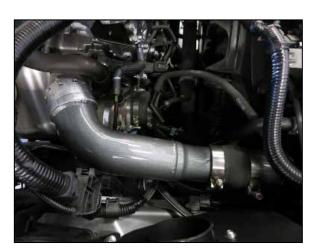
10. Install the K&N "Hot Side" charge tube into the coupler, then position the tube onto the turbo outlet and push the tube onto the outlet until an audible "click" is heard as the retaining clip locks onto the outlet. Position the tube and coupler for best fit and then secure the hose clamps.
