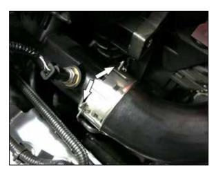
2. Release the retaining clip that secures the "Cold Side" charge tube to the intercooler and intake pipe on the engine by pushing the ears down into the locks on the coupler.
