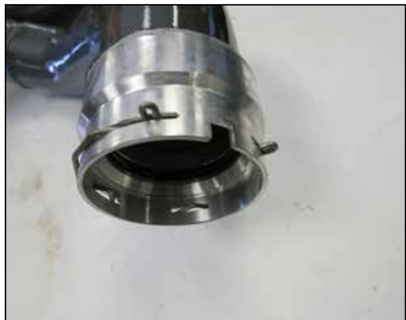
7. Remove the locking ring and O-ring from the factory charge tube coupler and install them into the K&N charge tube coupler. NOTE: The O-ring is directional, install it into the K&N charge tube the same direction it is installed into the factory charge tube.
