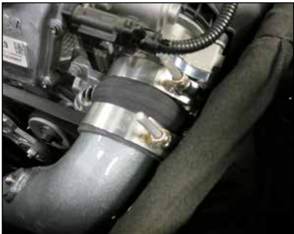
10. Install the K&N charge tube assembly and connect the intercooler connection and throttle body adapter. Push the intercooler connection until you hear the retaining clip audible "click" into its locked position. Position the hump coupler and secure with the provided hose clamps.
