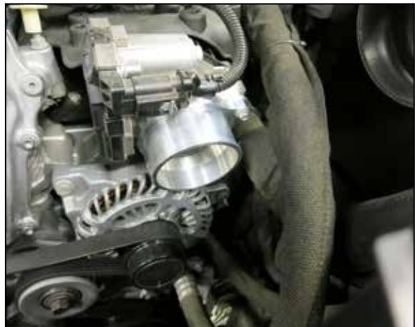
6. Install the K&N adapter onto the throttle body and secure with the factory bolts.
