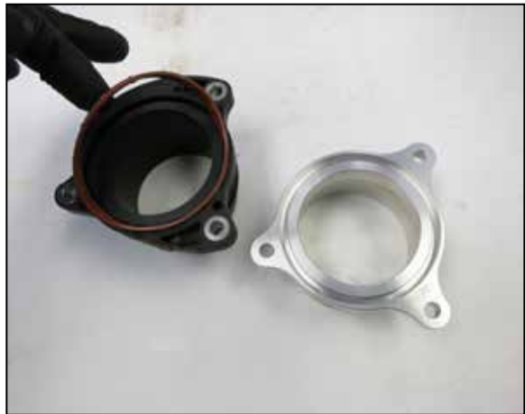
5. Remove the O-ring from the factory adapter and install it into the K&N adapter.
