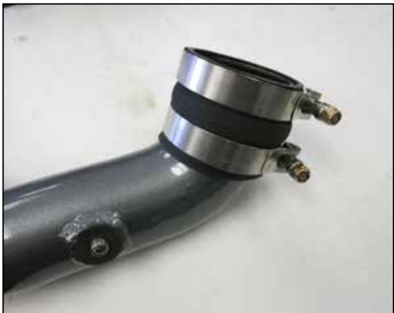
9. Install the hump coupler onto the K&N charge tube with the provided hose clamps. Do not tighten the hose clamps.
