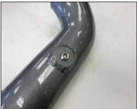
8. Install the 1/8" pipe plug into the accessory port of the K&N charge tube.
