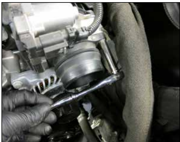
4. Remove the three bolts that secure the factory throttle body adapter to the throttle body and then remove the adapter.
