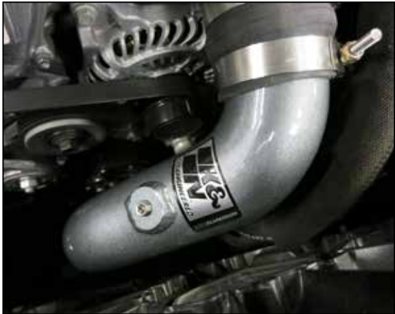
11. Apply the K&N decal onto the K&N charge tube as shown.
