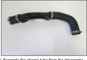
6. Separate the charge tube from the intercooler and throttle body and remove it from the vehicle.
