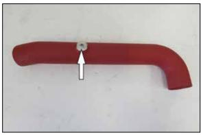
8. Install the provided NPT plug into the accessory port in the K&N charge tube.
