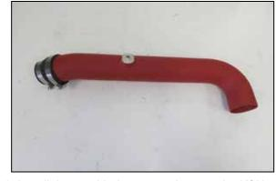
9. Install the provided step coupler onto the K&N charge tube and secure with the provided hose clamp.
