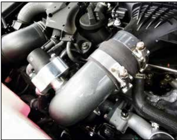
14. Install the passenger side K&N charge tube into the factory lower coupler, align with the upper hump coupler and install. Secure with the factory lower clamp and the upper hose clamp provided.
