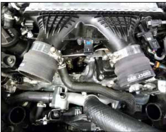
13. Install the provided hump couplers onto the intercooler and secure with the provided hose clamps.
