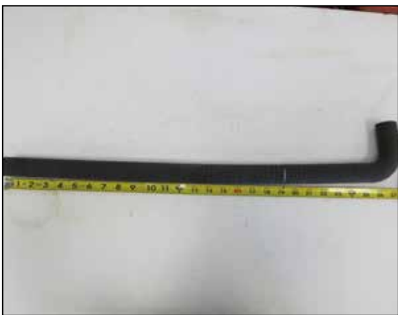
17. Cut the provided BOV hose at 19" as shown.
