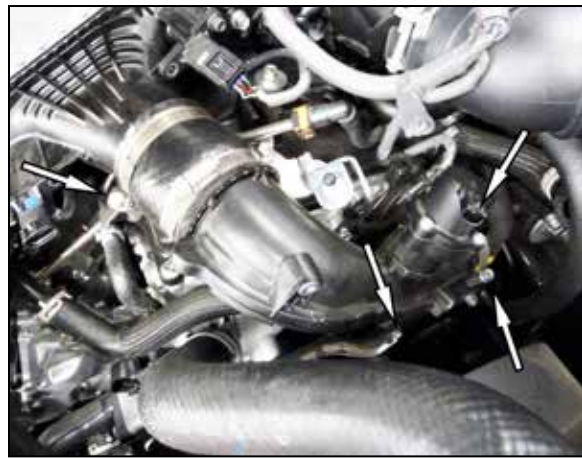
7. Disconnect the Driver side charge tube BOV electrical connection, remove the mounting bolt and loosen the hose clamps securing the driver side charge tube. Remove the driver side charge tube from the vehicle.
