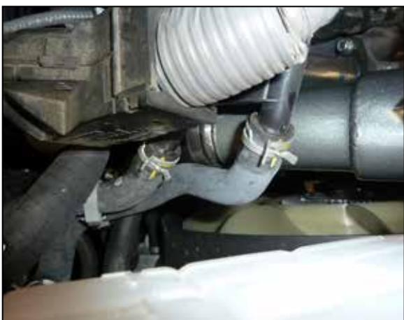
16. Rotate the heater hose spring clamps as shown to provide clearance for the BOV hose.
