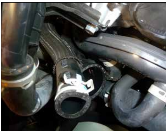
10. Release the clamp the secures the passenger side BOV hose and then remove the hose from the vehicle.
