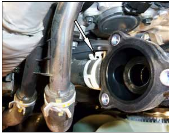
5. Release the spring clamp the secures the passenger side BOV hose to the charge tube and then disconnect the hose from the tube.
