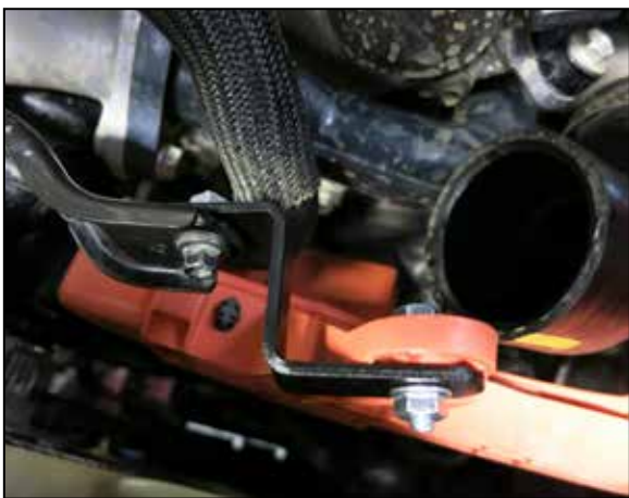
14a. On Hybrid models attach the provided "Z" bracket onto the factory harness bracket and then attach to the harness mount using the factory and provided hardware.
