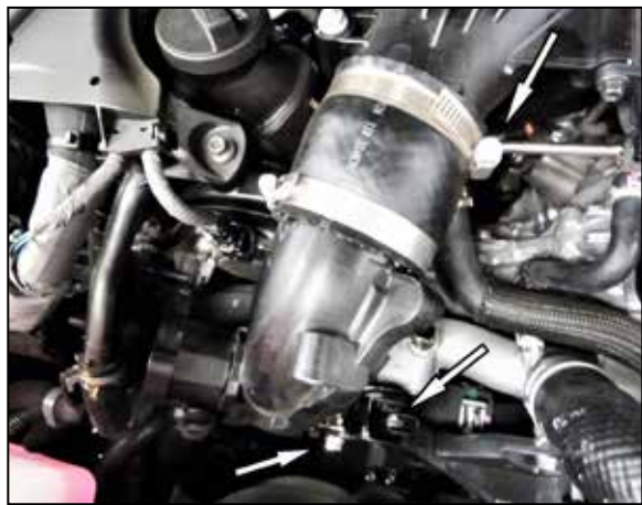
6. Remove the passenger side charge tube mounting bolt shown. Loosen the two hose clamps that secure the passenger side charge tube and then remove the charge tube from the vehicle. NOTE: ON Hybrid models the orange wiring harness holder will need to be removed from the factory charge tube.
