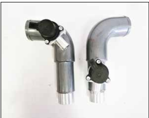
12. Install the BOV's onto the K&N charge tubes using the factory hardware.
