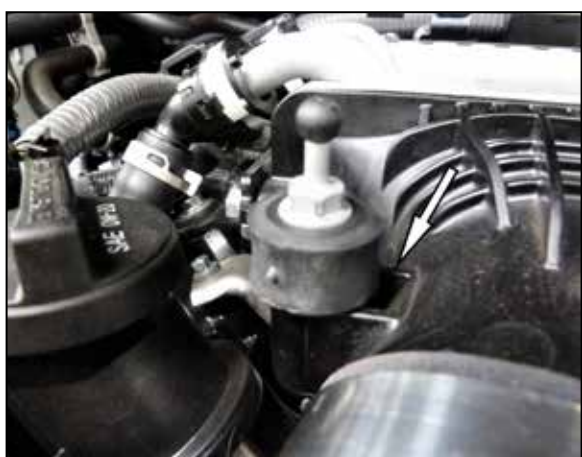
20. Remove the engine cover mounts, install the provided rubber mounts, and then reinstall the factory cover mounts.
