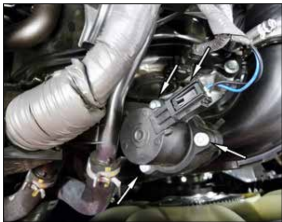
4. Disconnect the passenger side BOV electrical connection and then remove the three bolts securing the BOV to the factory charge tube. Remove the valve from the tube. NOTE: the bolts will be reused in a later step.
