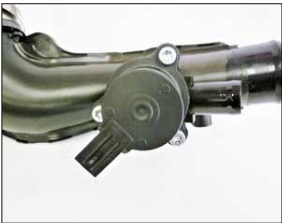
8. Remove the three bolts that secure the BOV to the driver side charge tube and then remove the valve. NOTE: These bolts will be reused in a later step.
