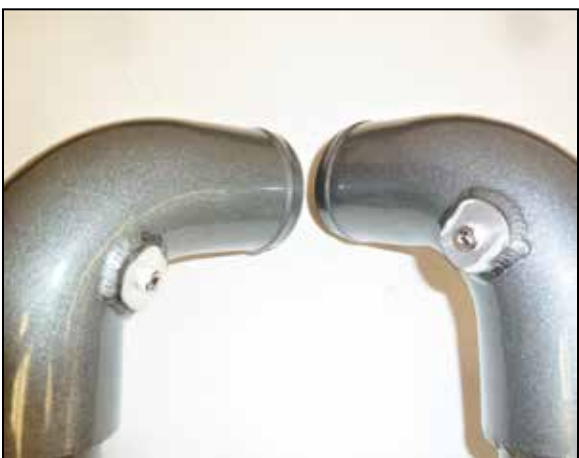
11. Install the 1/8npt pipe plugs into the accessory ports on the K&N charge tubes.
