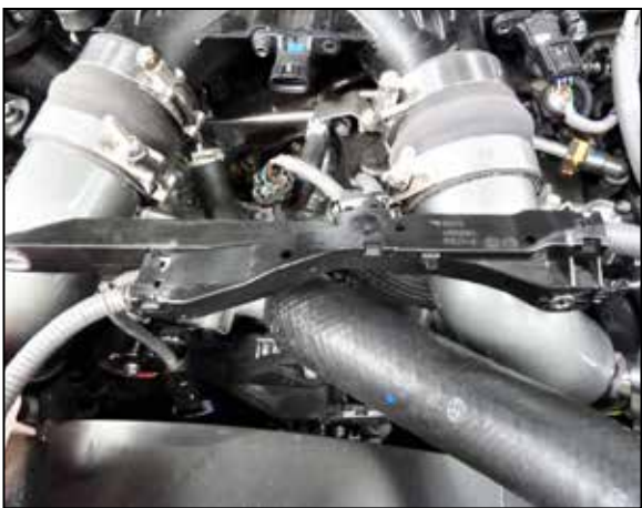
21. Unsnap and remove the plastic cover over the wiring harness.
