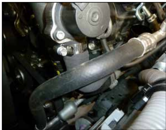
18. Install the shorter 90-degree section of BOV hose onto the driver side and secure with the provided clamps.
