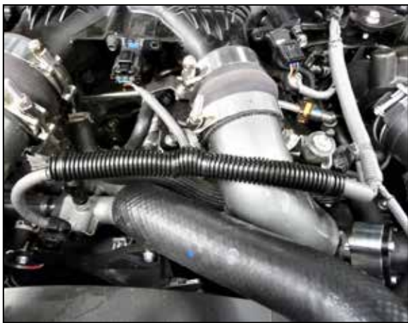
22. Install the provided corrugated harness cover onto the wiring harness.
