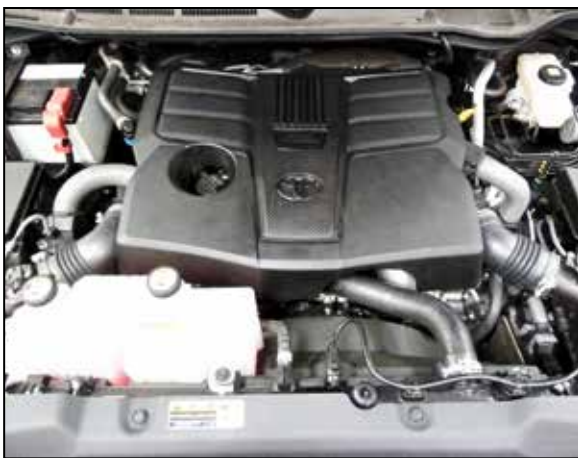
24. Reinstall the engine cover.
