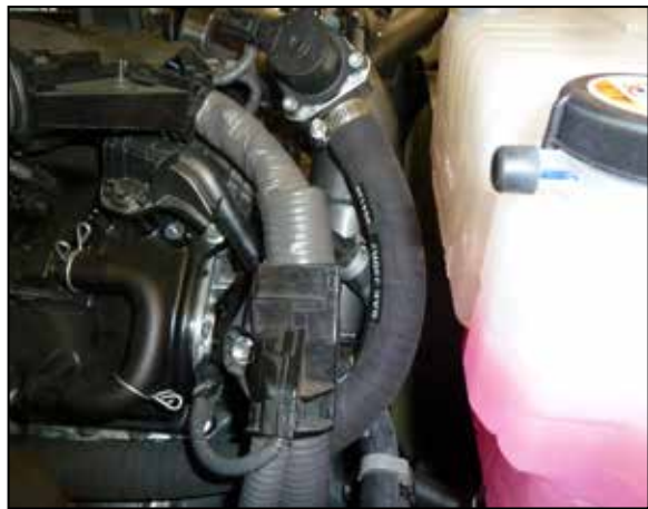
19. Install the longer BOV hose section onto the passenger side and secure with the provided clamps. NOTE: Double check the heater hose spring clamps will not cut the BOV hose. Reposition if necessary.
