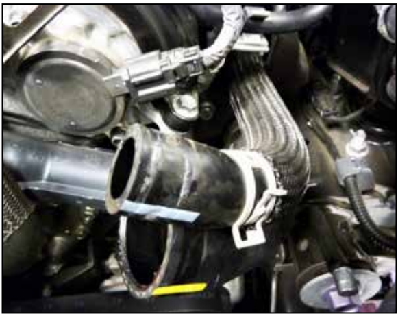
9. Release the clamp the secures the driver side BOV hose and then remove the hose from the vehicle.
