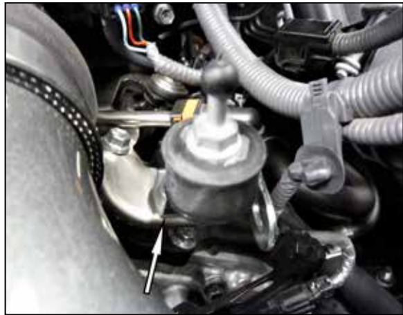
19. Install the longer BOV hose section onto the passenger side and secure with the provided clamps. NOTE: Double check the heater hose spring clamps will not cut the BOV hose. Reposition if necessary.
