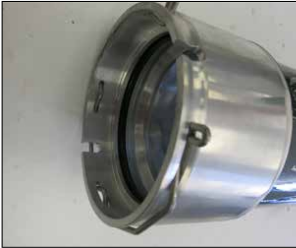
13. Install the O-ring and retaining clip into the K&N upper charge tube coupler. NOTE: Pay close attention to the direction of the lip seal position in the factory coupler and install it in the same direction into the K&N coupler.
