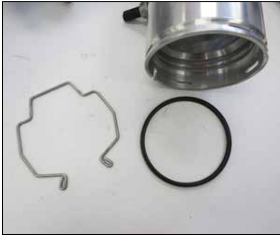
12. Remove the O-ring and retaining clip from the factory charge tube engine inlet coupler.
