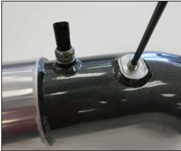
11. Install the 1/8 pipe plug into the accessory port.
