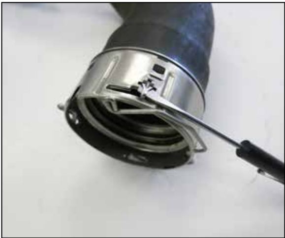
7. Release the tabs that retain the locking clip onto the factory intercooler coupler and then remove the clip from the coupler.
