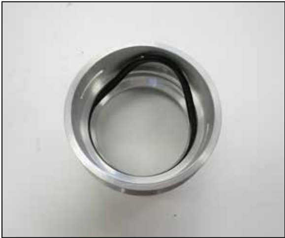
6. Remove the O-ring from the factory intercooler coupler and install it into the K&N coupler. NOTE: Pay close attention to the direction of the lip seal position in the factory coupler and install it in the same direction into the K&N coupler.
