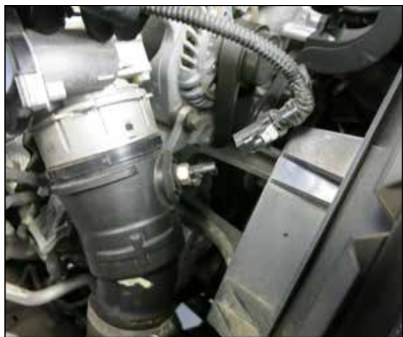
4. Disconnect the charge tube inlet temperature sensor electrical connection.
