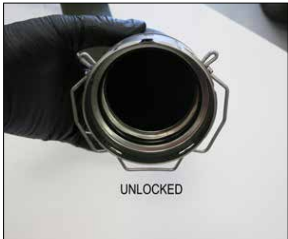
5. Release the retaining clips that secure the factory charge tube to the intercooler outlet and engine inlet by pulling them back. See photos. Remove the charge tube from the vehicle.
