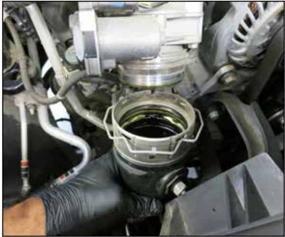
4. Disconnect the charge tube inlet temperature sensor electrical connection.
