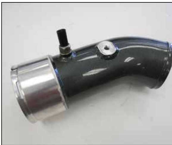
10. Remove the temperature sensor from the factory charge tube and install into the K&N upper charge tube.
