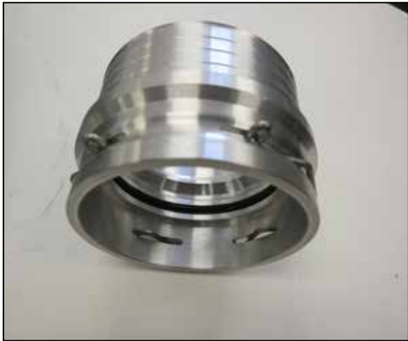
8. Install the locking clip onto the K&N intercooler coupler.
