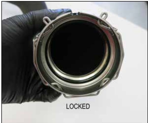
6. Remove the O-ring from the factory intercooler coupler and install it into the K&N coupler. NOTE: Pay close attention to the direction of the lip seal position in the factory coupler and install it in the same direction into the K&N coupler.
