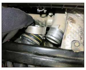
18. Separate the charge tube from the turbo and remove the clamp.
