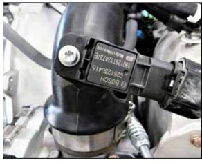
4. Remove the screw that secures the charge pipe pressure sensor, Remove the sensor from the charge tube and set on top of the engine to the side
