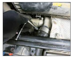
14. Loosen the hose clamp that secures the factory charge tube to the turbo outlet.
