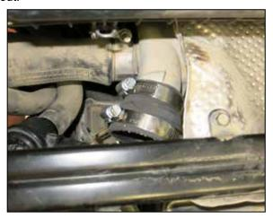
20. Install the step coupler onto the turbo outlet and secure with the provided hose clamp.
