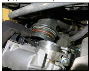
16. Separate the charge tube from the throttle body.
