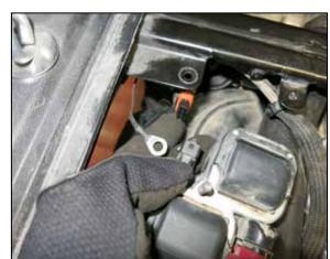
12. Pull back the coil and unhook the ground wire, remove the white plastic spacer, and disconnect the electrical connection and then set the coil aside.
