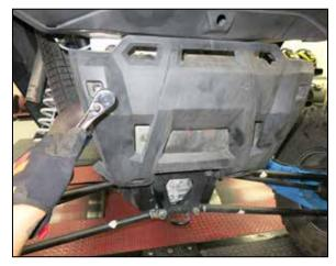
2. Remove the bolts that secure the exhaust system cover and then remove the cover and set aside.
