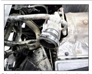
7. Install the step coupler onto the turbo outlet and secure with the provided hose clamp.
