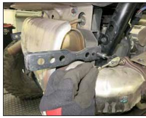
3. Remove the bolt that secures the muffler cover bracket to the chassis.
