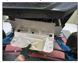
6. Remove the bolts that secure the muffler heat shield to the chassis and then remove the heat shield and set aside.
