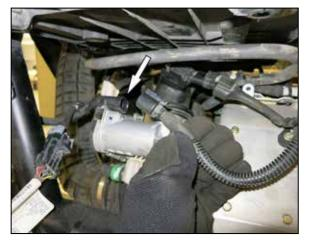
9. Disconnect the throttle body electrical connection
