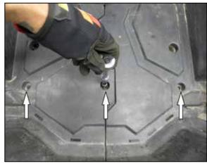
7. Remove the three bolts shown that secure the cargo bed to the support bracket.
