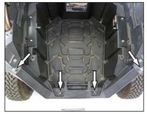
8. Remove the four bolts that secure the cargo box/ exhaust support bracket to the chassis and then remove the bracket and set aside.
