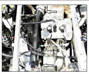
5. Loosen the two hose clamps that secure the charge tube to the turbo outlet and intake inlet, then remove the charge tube from the vehicle.
