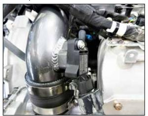
9. Install the charge pipe pressure sensor into the K&N charge pipe and secure with the provided hardware.
