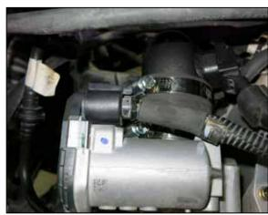
27. Reconnect the throttle body electrical connection.
