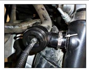
3. Pry up the tang to release the "one time use" hose clamp then separate the BOV valve from the charge tube.
