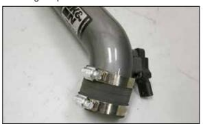
22. Install the provided straight coupler onto the K&N charge tube fully and do not tighten the hose clamp.
