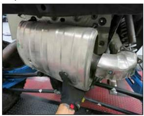
32. Reinstall the muffler using all of the factory hardware and springs.
