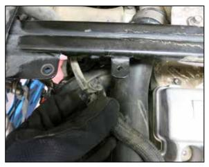
13. Sperate the vent line retaining clip from the chassis.
