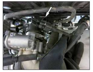
10. Disconnect the factory charge pipe pressure sensor electrical connection.
