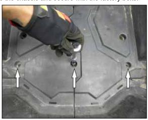
30. Reinstall the three-cargo box mounting bolts.
