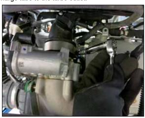
15. Loosen the hose clamp that secures the factory charge pipe to the throttle body.
