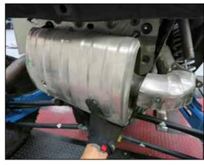
5. Remove the three nuts that secure the muffler to the exhaust pipe. Remove the mounting spring on the left side of the muffler and then remove the complete muffler assembly from the vehicle.
