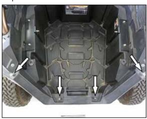
11. Reinstall the cargo box and secure with the factory hardware.
