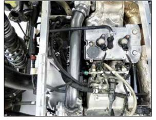
8. Install the K&N charge pipe into the couplers, adjust for best fit and then secure with the provided hose clamps.
