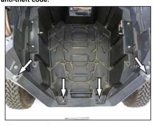
2. Remove the four bolts that secure the cargo box and then remove the cargo box from the vehicle.
