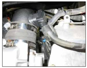
26. Reconnect the pressure sensor electrical connection.
