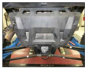
33. Reinstall the exhaust system cover over the muffler with the factory bolts.
