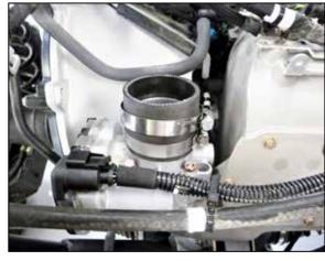
6. Install the straight coupler onto the throttle body and secure with the provided hose clamp.
