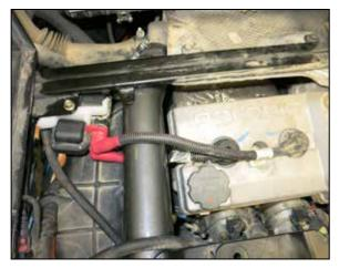
28. Reinstall the ignition coil using the factory hardware and spacer. **NOTE: The top spark plug wire will need to be routed over the top of the charge tube as shown.**
