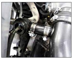
10. Using the provided coupler, connect the BOV to the charge tube and secure with the provided hose clamps.
