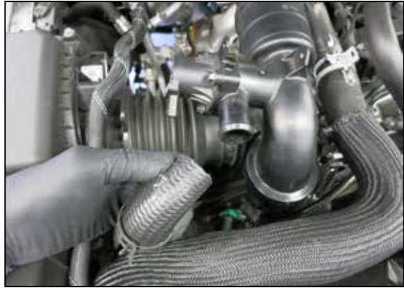
21. Release the spring clamp securing the BOV hose to the BOV and then disconnect the BOV hose.
