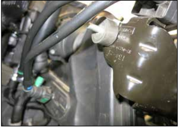
26. Install the provided rubber mounted stud onto the charge tube mount.
