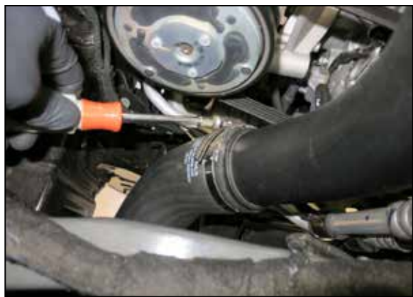
19. Loosen the hose clamp that secures the hot-side charge tube to the intercooler inlet hose.
