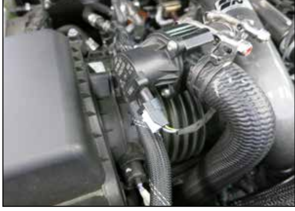
30. Reconnect the BOV valve electrical connection.
