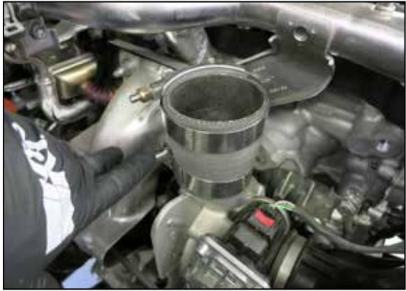
25. Install the provided step hose onto the turbo outlet and secure with the provided hose clamp.
