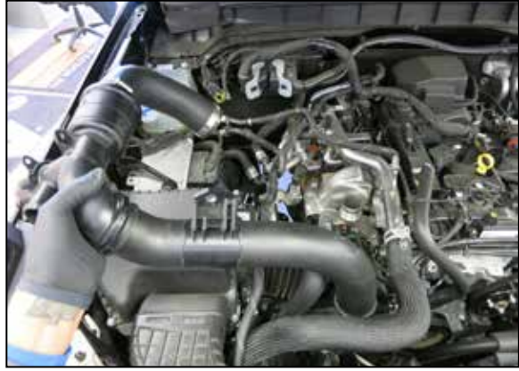
22. Remove the hot-side charge pipe from the vehicle.
