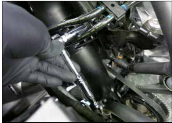
20. Remove the bolt that secures the charge tube to the mount.
