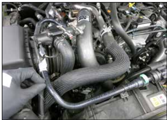
31. Reinstall the CCV hose to the quick connect fittings. Install the K&N decal as shown.
