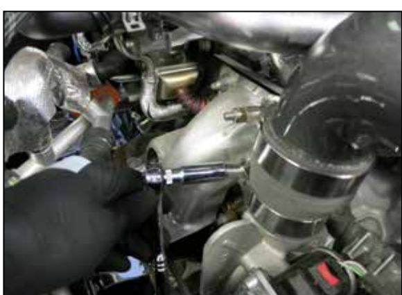
24. Remove the BOV from the factory charge tube and install it onto the K&N BOV manifold using the provided hardware.
