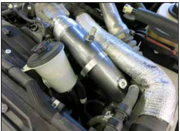
13. Install the K&N charge tube into the vehicle so the tube engages into the elbow coupler. NOTE: Apply spray lube to the tube/elbow connection to aid the insertion of the tube into the coupler as it is a tight fit.
