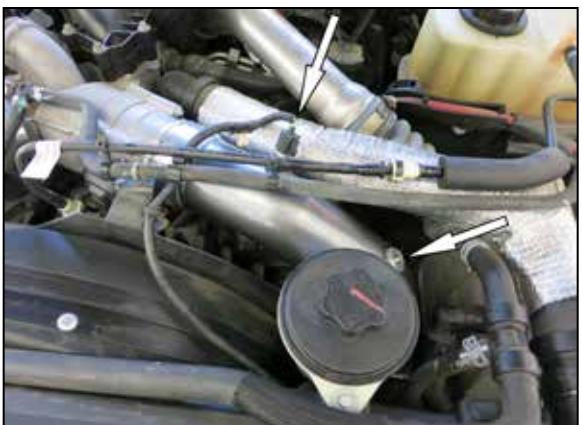
17. Reconnect the IAT sensor electrical connection and position the vent lines and harness.
