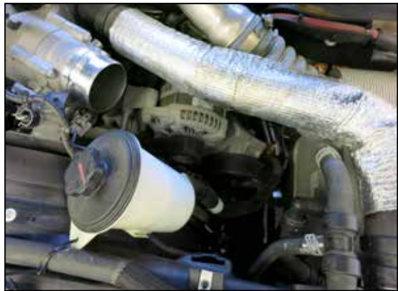
9. Remove the bolt that secures the power steering reservoir and set the reservoir to the side to aid with clearance during installation of the K&N charge tube.
