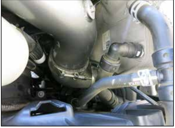
15. Adjust the tube and elbow coupler for best fit and then secure the hose clamps.
