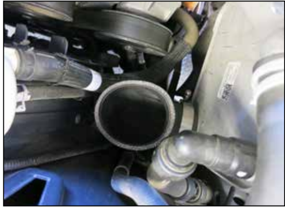
10. Install the provided elbow coupler onto the intercooler with the provided clamp but do not tighten completely.
