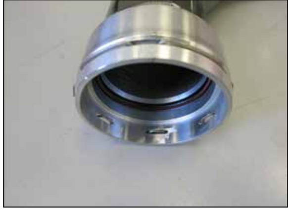
12. Remove the O-ring and retaining clip from the factory charge tube and install them into the K&N charge tube.
