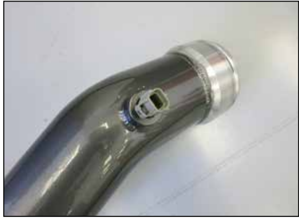
11. Remove the IAT sensor from the factory charge tube and install it into the K&N charge tube.
