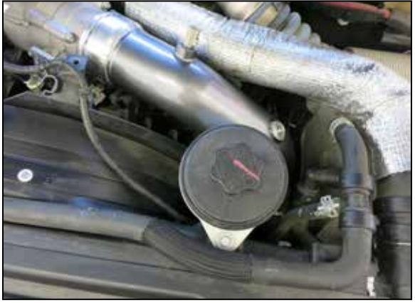
16. Reinstall the power steering reservoir and secure with the factory bolt.
