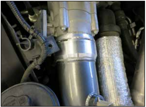
14. Connect the quick connector to the throttle body, push the coupler firmly until there is an audible "click" is heard. Pull back on the coupler to be sure the locking ring is engaged.
