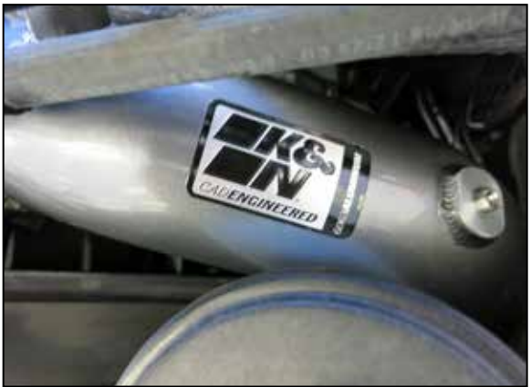
18. Install the provided 1/8" npt plug and K&N decal. Be sure to apply thread sealer to the npt threads.
