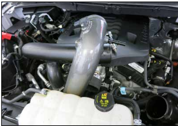
17. Feed the K&N charge tube into position from the top of the engine compartment. Adjust the 90deg hose so that the charge tube inserts into the hose.
