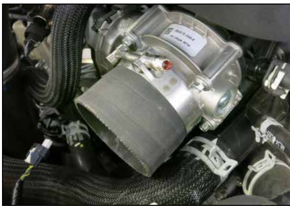
15. Install the provided step hose onto the throttle body and secure with the provided clamp.
