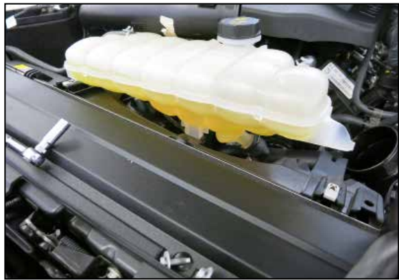
6. Remove the two bolts that secure the coolant reservoir, this will allow the reservoir to be moved to allow easier access while working on the lower section of the charge tube.
