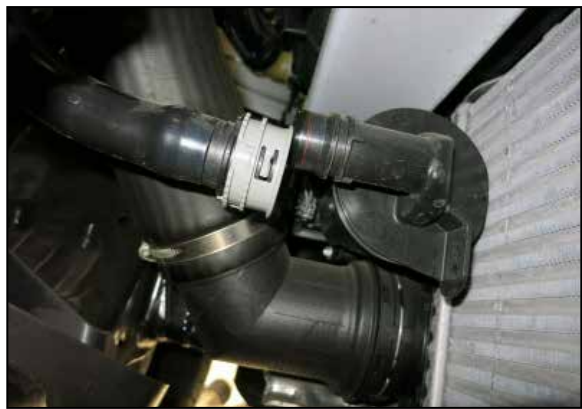
7. Rotate the BOV locking ring counterclockwise to unlock and then separate the BOV hose from the fitting.
