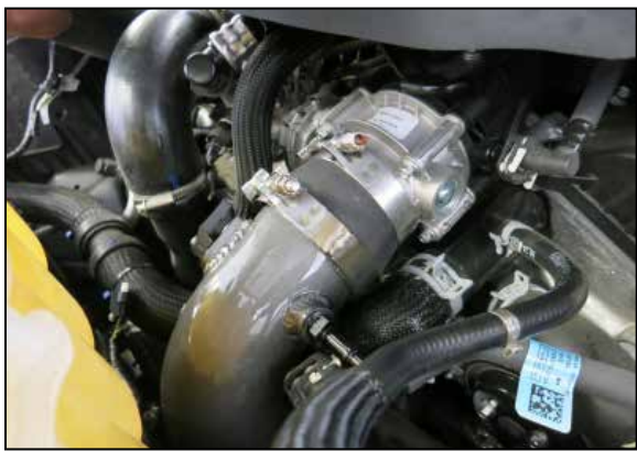
18. Position the tube into the hose at the throttle body, adjust the entire assembly for best fit and then secure the hose clamps. Reconnect the BOV hose onto position and lock by turning the locking ring clockwise.
