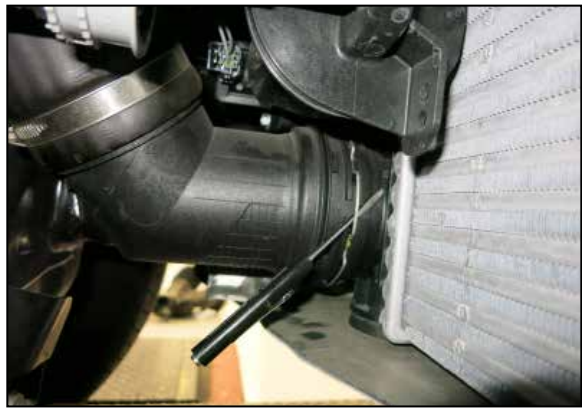
8. Using a small screwdriver or similar tool, release the locking clip that secures the factory charge tube to the intercooler and then disconnect the tube from the intercooler connection.
