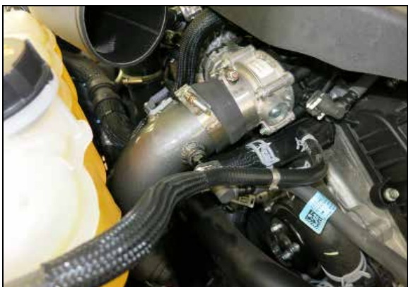
22. Reinstall the intake tube and secure with the factory clamps.
