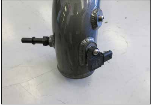
14. Remove the Pressure sensor from the factory charge tube and then install it into the K&N charge tube using the provided hardware. Install the quick connect npt fitting into the K&N charge tube and then install the 1/8npt plug. Be sure to apply thread sealant to the threads of the 1/8npt plug before installing.
