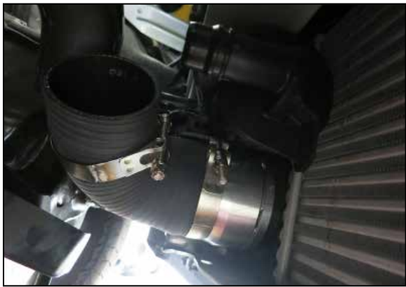
16. Install the quick connector/90deg. hose assembly onto the intercooler, push the connector firmly onto the intercooler until you hear an audible click indicating the locking ring has snapped into position.
