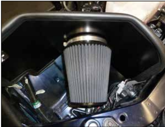
24. Install the K&N air filters onto the filter adapters and secure with the provided hose clamp.
