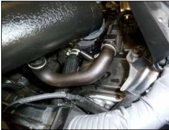
22. Connect the passenger side PCV hose to the fitting installed into the intake tube and secure with the factory spring clamp.
