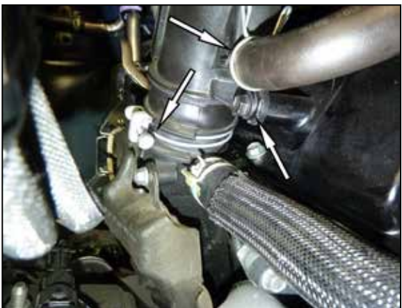
5. Disconnect the PCV hose from the passenger side lower intake tube, Remove the intake tube mounting bolt then loosen the hose clamp securing the intake tube to the turbo inlet and remove the tube from the vehicle.
