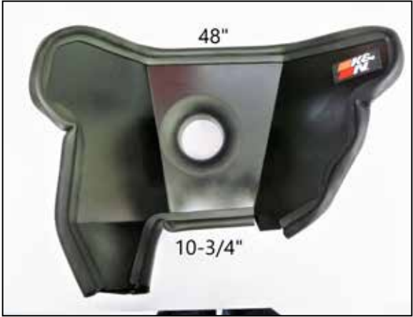
11. Cut the 61" edge trim to lengths of 10.75" and 48", install the edge trim onto the driver side heat shield as shown.
