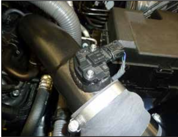
22. Connect the passenger side PCV hose to the fitting installed into the intake tube and secure with the factory spring clamp.
