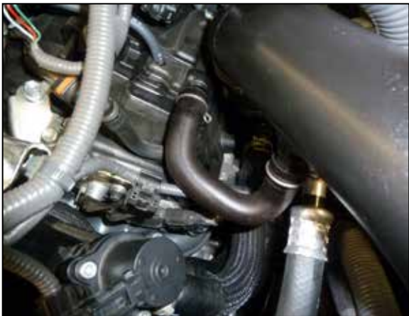
21. Connect the driver side PCV hose to the fitting installed into the intake tube and secure with the factory spring clamp.
