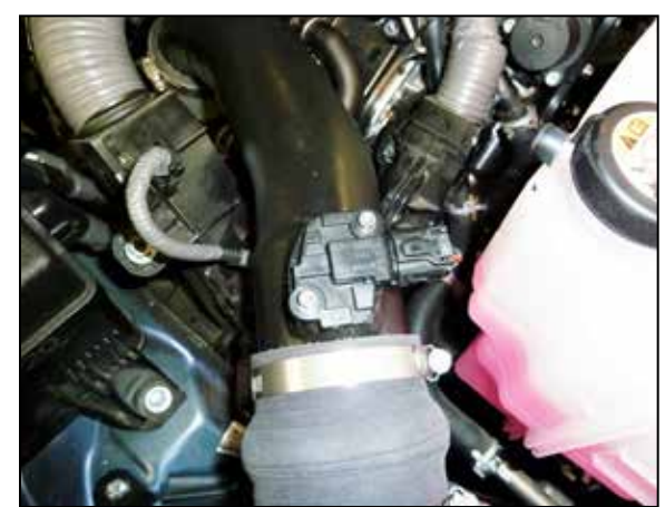
23. Reconnect the mass air sensor electrical connections.
