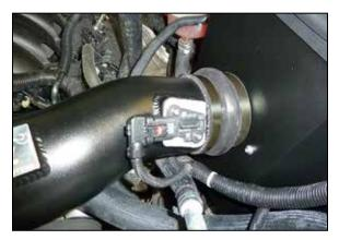
25. Connect the mass air sensor electrical connection.
