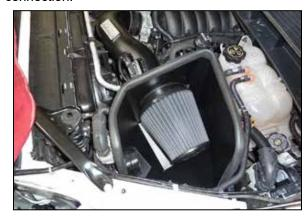
26. Install the K&N® air filter onto the adapter and secure with the provided hose clamp.
