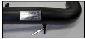
15. Install the quick connect fitting into the  $K\&N^{\otimes}$  intake tube as shown.
