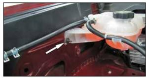
11. Remove the nut that secures the coolant reservoir to the inner fender.
