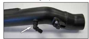
14. Install the  $90^{\circ}$  vent fitting into the K&N<sup>®</sup> intake tube as shown.
