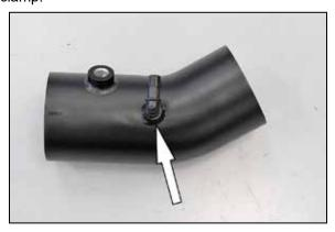
15. Install the provided 90° NPT vent fitting into the K&N® intake tube as shown.
