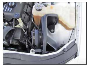
13. Set the heat shield assembly into position in the engine bay so the inserted nut passes into the air box mounting hole in the inner fender. Do not secure the heat shield at this time.
