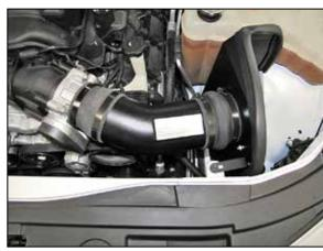
18. Install the K&N® intake tube into the silicone hump hose and then into the into the silicone step hose at the throttle body. Align the intake tube and heat shield for proper fit and then secure the intake tube with the provided hose clamps and the heat shield bracket with the factory air box retaining bolt removed in an earlier step.
