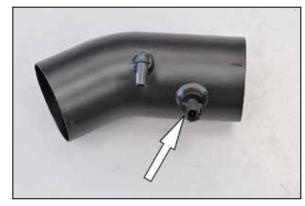
17. Install the inlet air temperature sensor into the  $K\&N^{\otimes}$  intake tube as shown.
