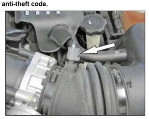
2. Disconnect the inlet air temperature air sensor electrical connection.
