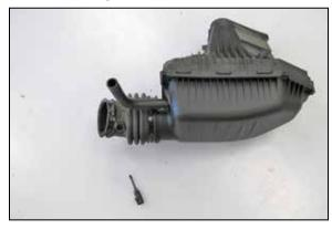
16. Remove the inlet air temperature sensor from the factory intake tube as shown.
