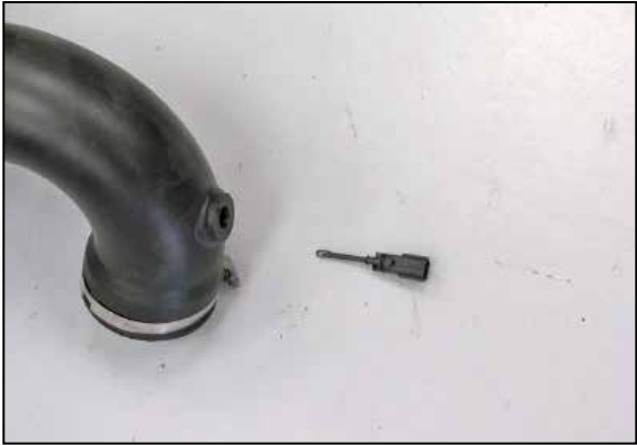
24. Remove the inlet air temperature sensor from the factory intake tube as shown.
