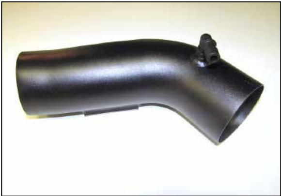
23. Install the vent fitting into the K&N® intake tube as shown. NOTE: NPT fittings are easy to cross thread. Install the vent fitting “hand” tight, then turn it two complete turns with a wrench.
