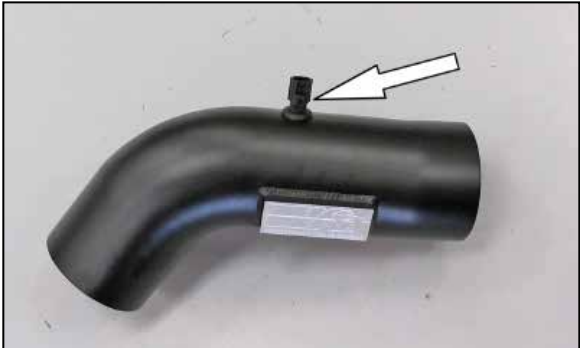
25. Install the inlet air temperature sensor into the grommet installed into the K&N® intake tube as shown.
