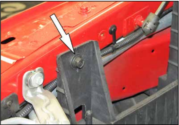
18. Remove the front air box mounting bracket bolt shown. NOTE: This bolt will be reused in a latter step.
