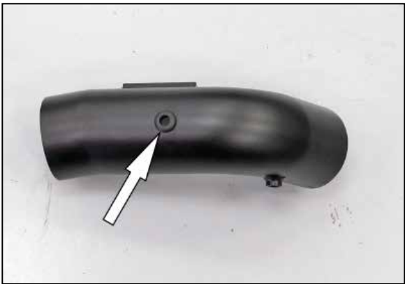
22. Install the provided grommet into the K&N® intake tube as shown.
