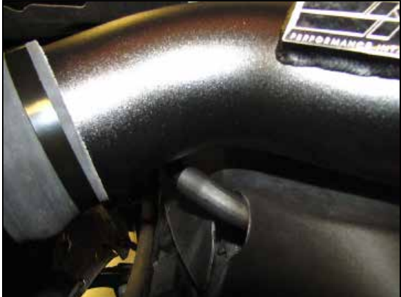
27. Connect the crank case vent hose to the fitting installed into the K&N® intake tube and secure with the provided hose clamp. NOTE: Some trimming of the vent hose will be necessary. NOTE: If the vent hose kinks, use the provided 90° fitting and additional hose clamps to route the hose free of kinks.
