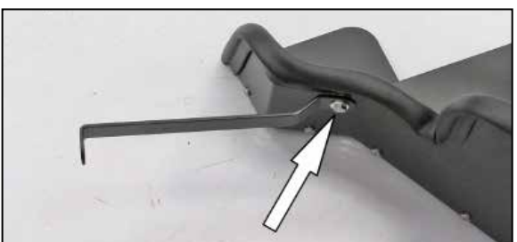
17. Install the heat shield mounting bracket (083103-1A) onto the heat shield using the provided hardware. NOTE: Do not completely tighten at this time. NOTE: When using the cut out heat shield wall, place the provided spacer between the bracket and heat shield and use the longer bolt.
