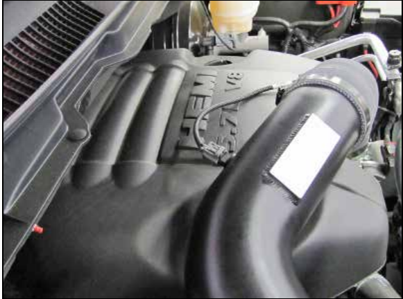
28. Choose the appropriate inlet air temperature sensor extension harness and then connect Install it too the inlet air temperature sensor and vehicle harness. NOTE: The vehicle manufacturer uses two different inlet air temperature sensor connections, choose the correct extension harness for the sensor provided by the manufacturer. Secure the harness with the provided tie wrap.
