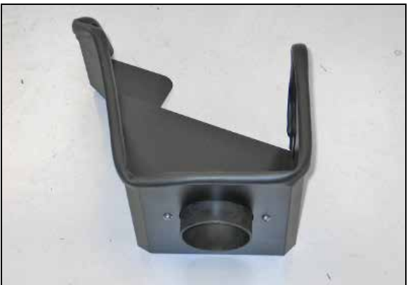
14. Install the provided filter adapter into the K&N® heat shield and secure with the provided hardware.
