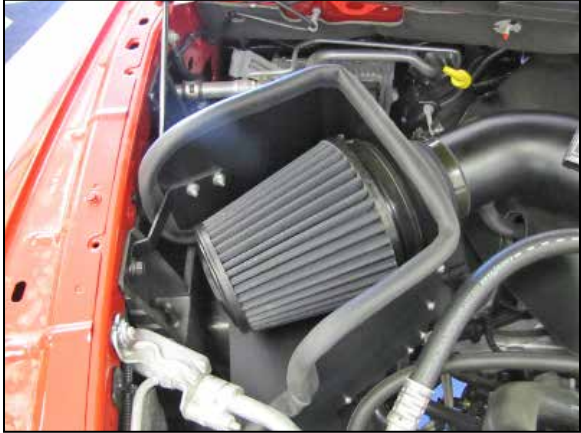
29. Install the K&N® air filter and secure with the provided hose clamp.
