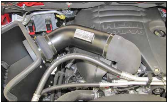
26. Install the K&N® intake tube into the silicone hump hose and then align with the hose on the throttle body. Align the hose, tube and heat shield for proper fit and then secure with the provided hardware.
