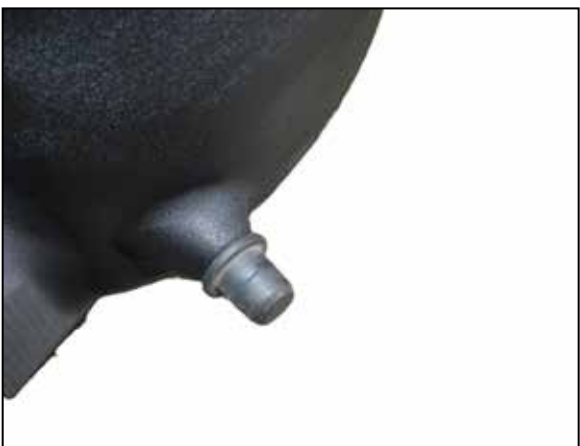
11. Remove the factory rubber isolator from the OEM air box and attach to the mount on K&N airbox like image shown.
