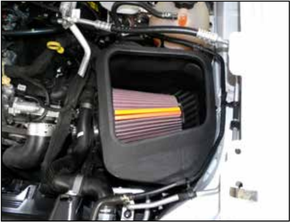
12. NOTE: Pre-assembled from the factory. Remove K&N Filter from airbox, Remove filter cap. Install the K&N air filter housing assembly into the vehicle and position to OEM air box locations. Secure using OEM bolt.
