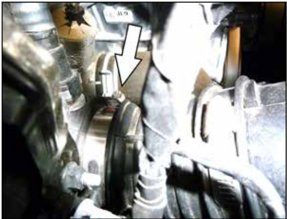
5. Loosen the clamp on the turbo using 7mm socket or nut driver. Also, loosen the clamp on the air box.
