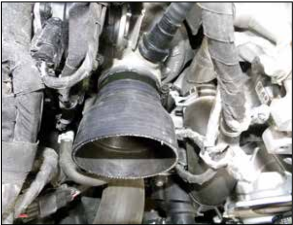
14. NOTE: Pre-assembled from the factory. Install the step hose with clamps to the turbo tighten clamp on the turbo only.
