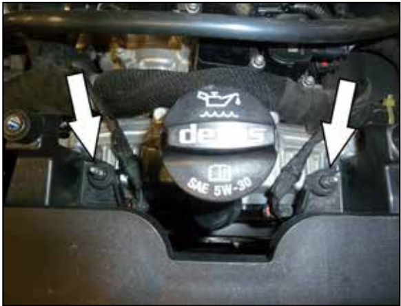
7. Locate the 2 nuts holding in the intake tube. Loosen using 10mm socket and remove.
