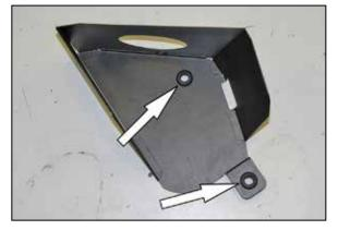
5. Install the two provided grommets into the heat shield as shown.
