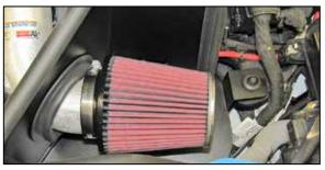
20. Install the K&N® air filter onto the intake tube and secure with the provided hose clamp.
