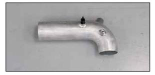
13. Install the provided vacuum fitting into the K&N® intake tube as shown.
