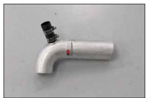
15. Install the secondary air fitting onto the K&N<sup>®</sup> intake tube as shown.
