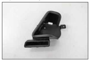
10. Install the fresh air intake scoop into the heat shield assembly as shown.
