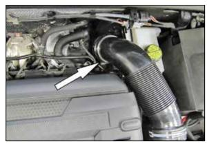
2. Loosen the hose clamp that secures the intake tube to the turbo inlet.
