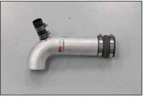
16. Install the remaining coupling hose (08185) onto the K&N<sup>®</sup> intake tube as shown.
