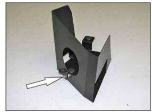
6. Install the provided tube mounting bracket (064314) onto the heat shield as shown.
