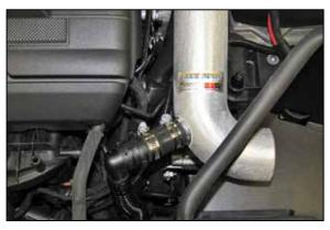
19. Connect the secondary air hose onto the Quick disconnect fitting and connect the vacuum line to the fitting installed into the K&N® intake tube.
