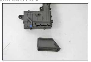
9. Remove the fresh air intake scoop from the factory air filter housing.
