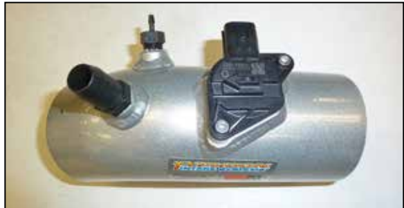
8. Remove the mass air sensor from the factory housing and install it into the K&N® intake tube and secure with the provided hardware.
