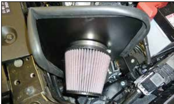
16. Install the K&N® air filter onto the filter adapter and secure with the provided hose clamp. NOTE: Drycharger® air filter wrap; part # RU-5147DK is available to purchase separately. To learn more about Drycharger® filter wraps or look up color availability please visit http://www.knfilters.com ®.
