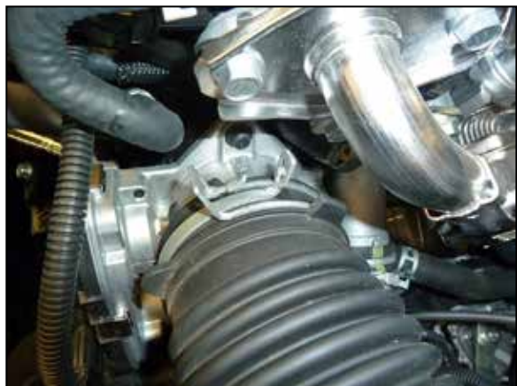
5. Release the spring clamp for the intake hose at the throttle body and then disconnect intake hose from the throttle body.
