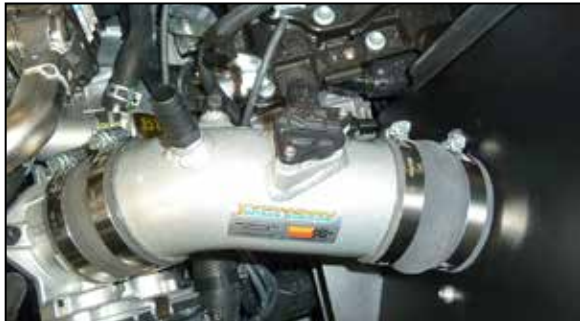
17. Install the K&N® intake tube assembly into the couplers and adjust for best fit and secure with the provided hose clamps.
