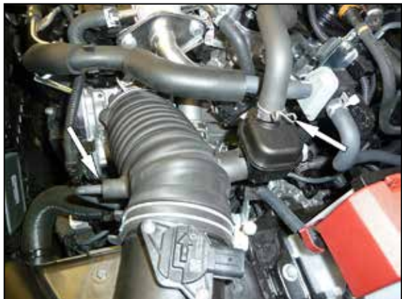
4. Disconnect the Crank case vent line and small vent line shown.
