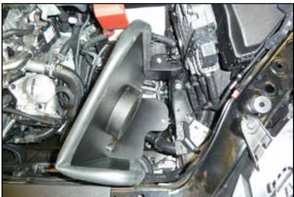
13. Install the heat shield into the vehicle so the mounting posts insert into the factory grommets.
