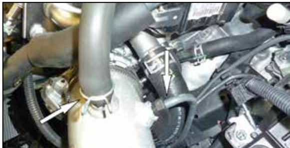
18. Connect the crank case vent line and vacuum line to the vent fittings installed into the K&N® intake tube.
