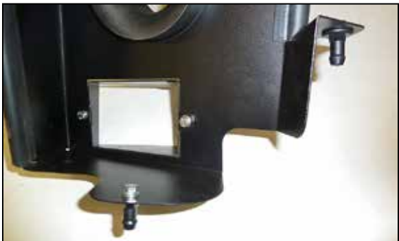
12. Install the two mounting posts onto the heat shield as shown using the provided hardware.
