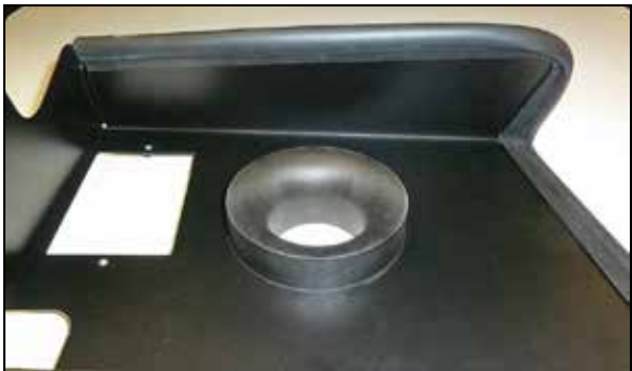
10. Install the filter adapter into the heat shield and secure with the provided hardware.
