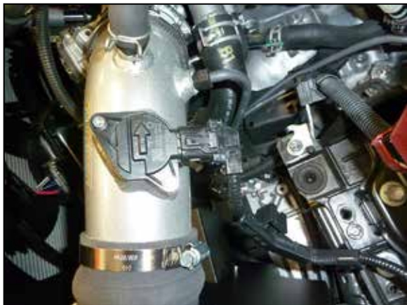
19. Reconnect the mass air sensor electrical connection.
