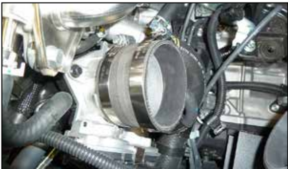
15. Install the provided straight coupler (08711) onto the throttle body and secure with the provided hose clamp.
