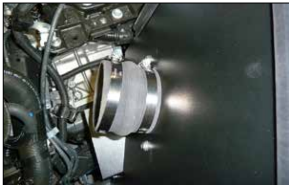
14. Install the provided hump coupler (087121) onto the filter adapter and secure with the provided hose clamp.
