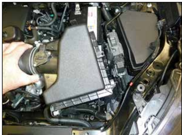
6. Pull upwards on the air box assembly and remove it from the vehicle. NOTE: K&N Engineering, Inc., recommends that customers do not discard factory air intake.
