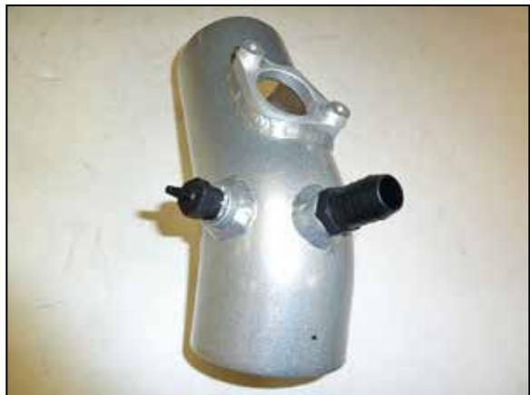
7. Install the provided vent fittings into the K&N® intake tube as shown. NOTE: NPT fitting has tapered threads and only designed to be installed until hand tight, then tighten one rotation or when the fitting becomes difficult to return.
