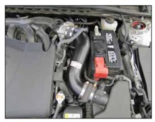
7. Install the K&N® intake tube into the coupler at the throttle body and then into the coupler at the air filter housing, adjust the tube for best fit and then secure with the provided hose clamps. Connect the crank case vent line to the fitting installed into the K&N® intake tube.
