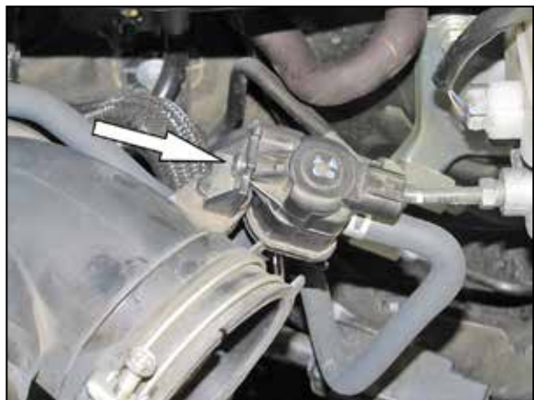
8. Unbolt the EVAP solenoid from the mounting bracket.
