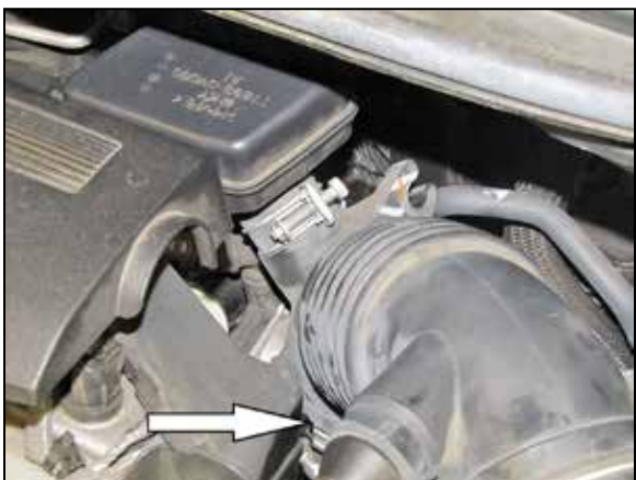
9. Loosen the hose clamp securing the intake hose to the throttle body and remove the intake hose from the vehicle.
