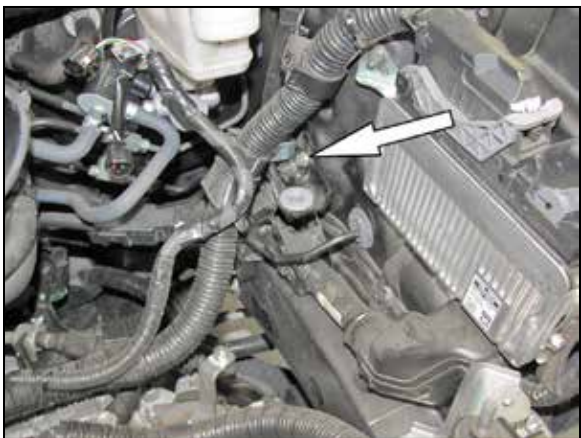
10. Remove the bolt securing the rear air box mounting bracket to the strut tower and then remove the bracket from the strut tower.
